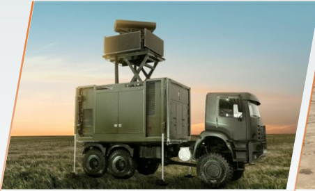
M200 VIGILANTE Medium-Altitude Air Defense • 3D radar • Electronic Scan • 200 km range • Integrated IFF
