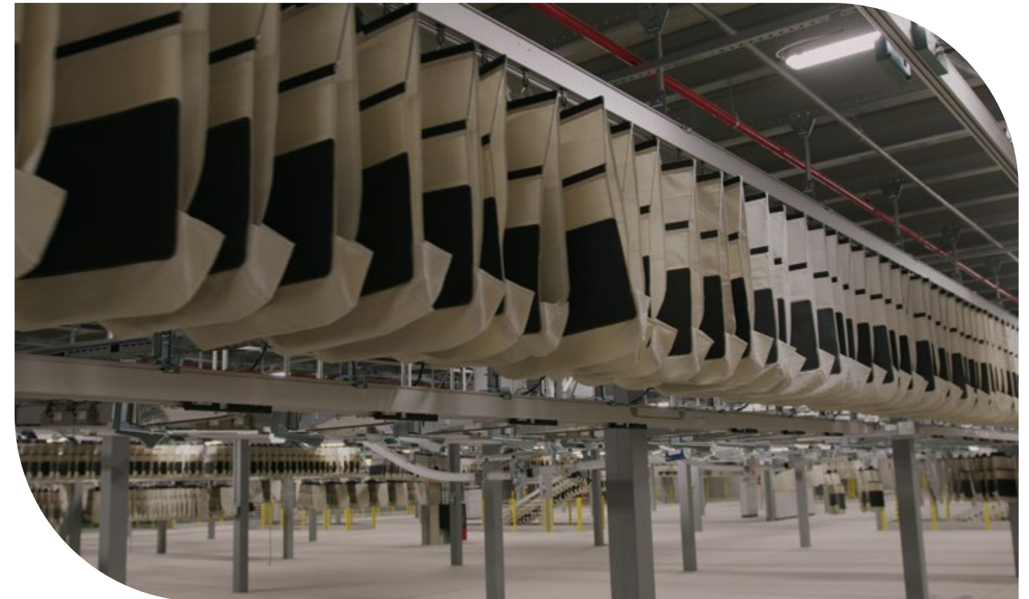
Automated order separation at our DC in Cabreúva (SP).
