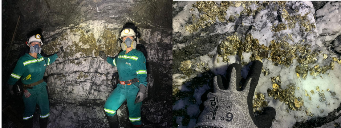
Figure 7-7: A) Sulfide-rich laminated quartz vein in the Matinha body. B) Detailed pyrite crystals in the Matinha body (NX Gold, 2023)
