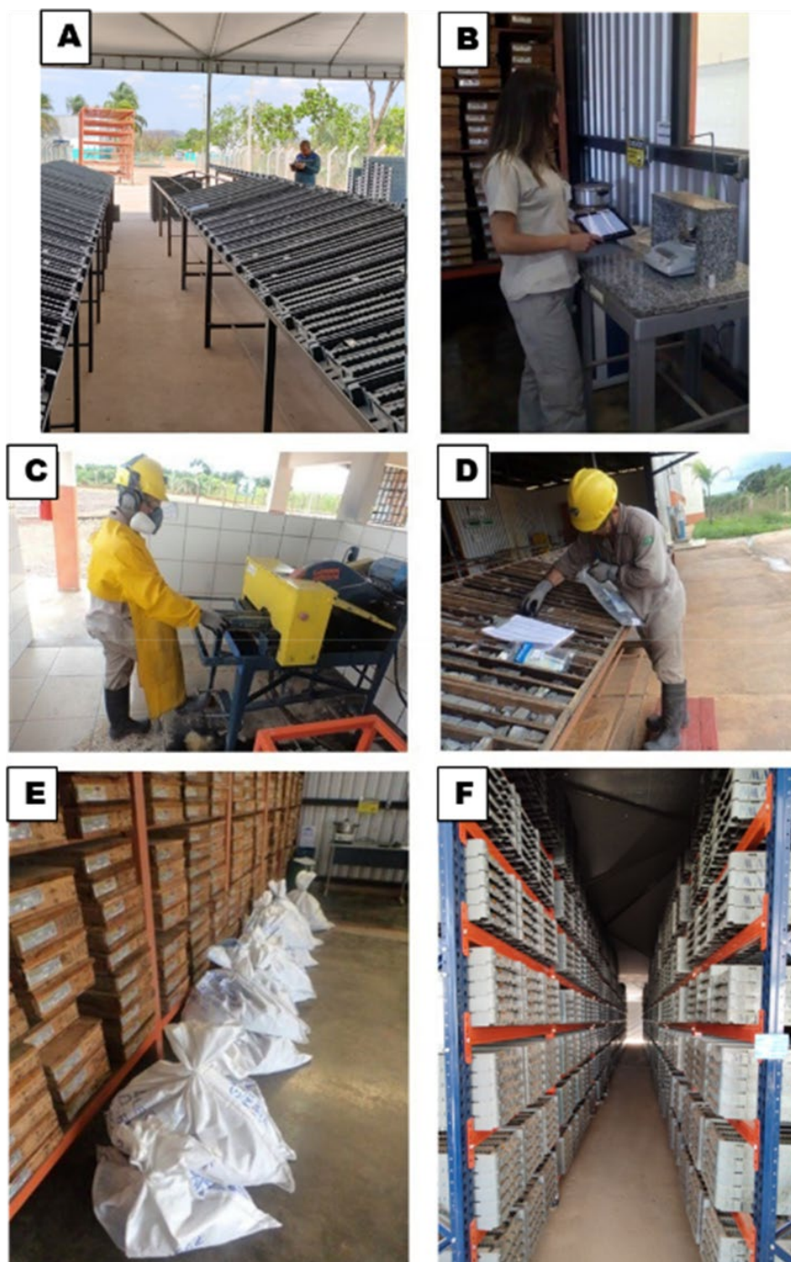
Figure 11-2: Photographs of standard operating procedures: (A) Geological and geotechnical core logging, sample selection for laboratory analysis; (B) density measurements ; (C) drill core cutting; (D) sampling of sawn core; (E) sample batch preparation for laboratory transfer; (F) core box storage (NX Gold, 2022)
