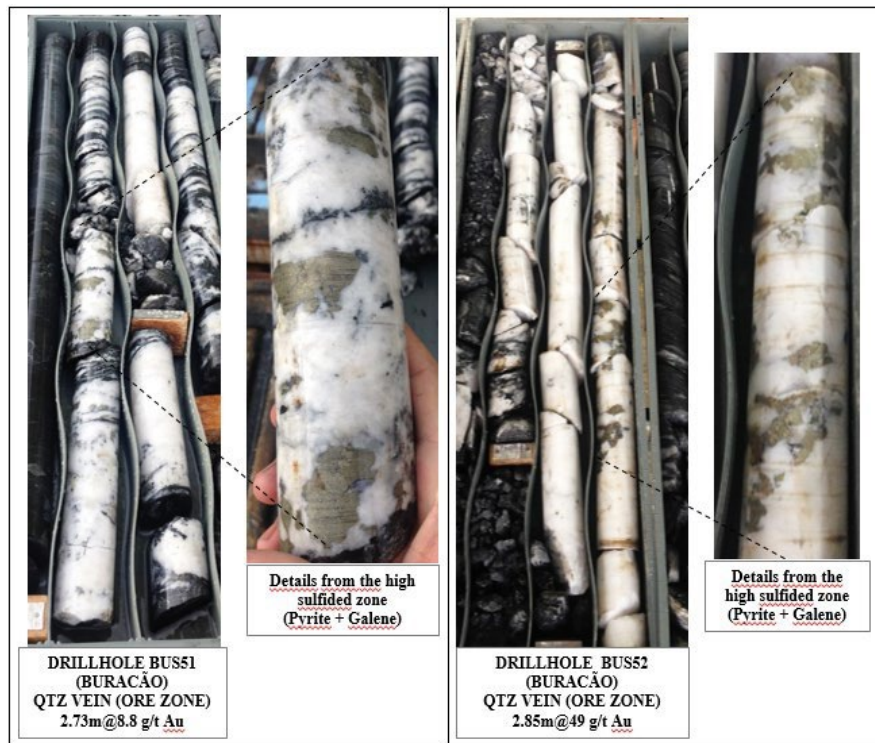
Figure 7-8: Quartz vein with high sulfidation (Pyrite and Galena) and high gold grade (NX Gold, 2018)
