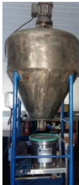
Figure 13-5: Falcon Concentrator L40 - Laboratory Size
