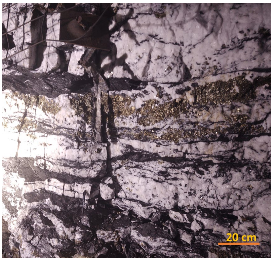
Figure 12-3: Data verification: Sulfide quartz vein in underground mine (September 2025)
