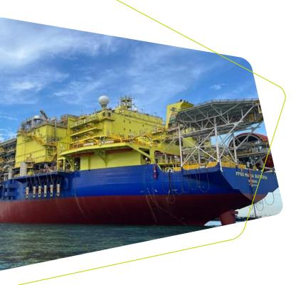
In addition, FPSO Maria Quitéria left the shipyard in China in May 2024. This platform will operate in the Jubarte field, located in Campos Basin presalt, on the coast of Espírito Santo, and has decarbonization technologies, such as the combined cycle in power generation and the Flare Gas Recovery Unit - FGRU (closed flare). Its production capacity is 100 Mbpd of oil and 5 MMm³/d of natural gas.
