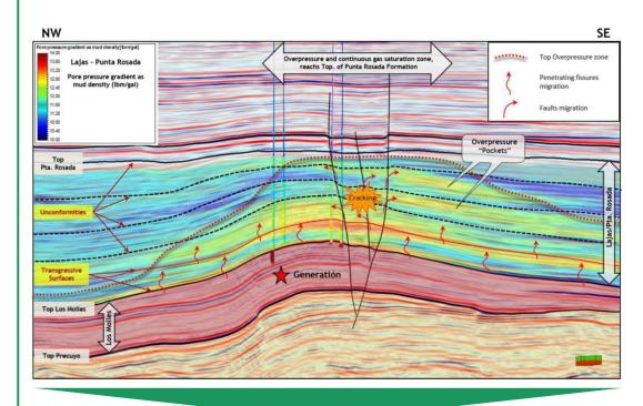
NW-SE Seismic section with calculated Pore Pressure Gradient, illustrating the play concept of Rio Neuquén Gas Field proved by the RN.x-2100 exploratory well, drilled in 2021 in Rio Negro Province
