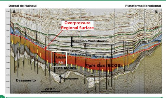
The proven model of accumulation in the Neuquén Basin is **unconventional**, known as **Basin-centered gas**. It is characterized by the absence of a conventional sealing rock as the upper limit of the accumulation. Instead, this limit is represented by an irregular level of overpressure on a basin and block scale, configuring a **hydrodynamic seal in rocks with very low permeability** in the Punta Rosada and Lajas Formations
