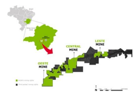
Mineração Usiminas operates one crushing/classification plant located in the Leste mine, and three concentration plants located in the Oeste and Central mines. Its major processing facilities include crushers, mill, screens, cyclones, spiral classifier, spiral concentrators, jigs, magnetic concentrators, flotation cells, flotation columns, filters and a decanter.
