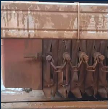
Dewatering ultrafine tailings requires filter press technologies.
