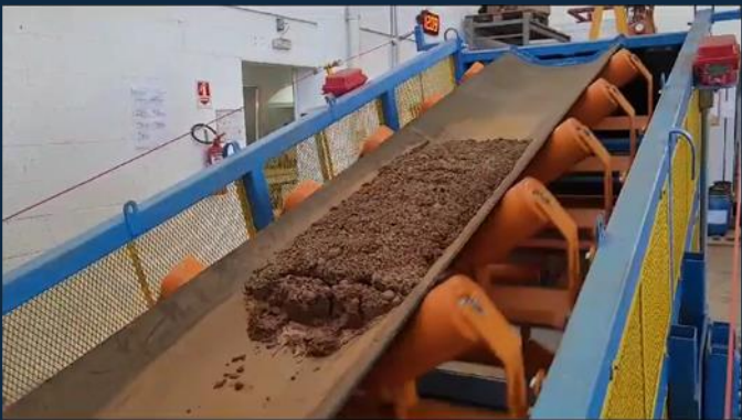
Ultrafine tailings' moisture and granulometry brings additional challenges to long distance conveyor belts .
