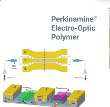
**Electro-Optic Polymer slot modulators**
