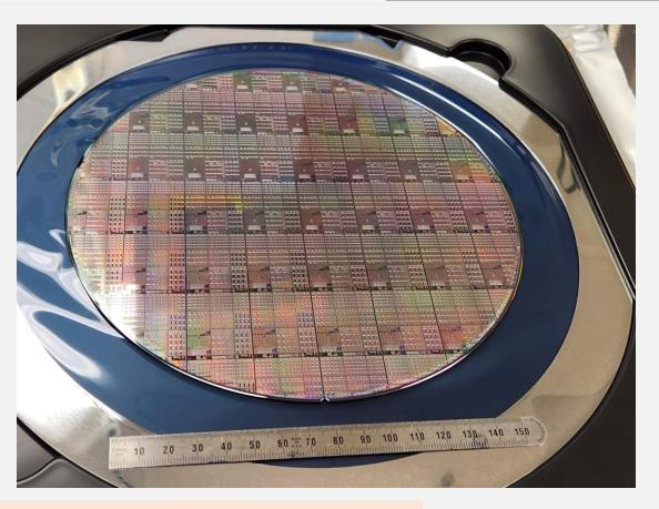
Volume scale silicon slot designs on 200mm wafers
