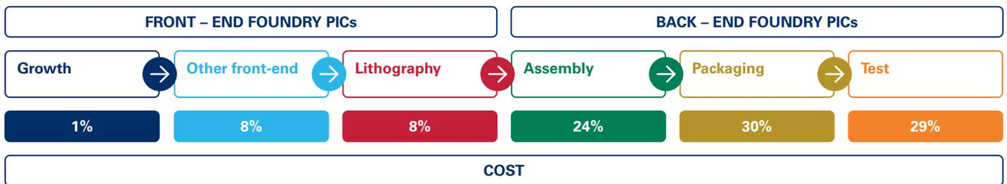
Figure 18 Break-out of the cost for a PIC module<sup>15)</sup>
