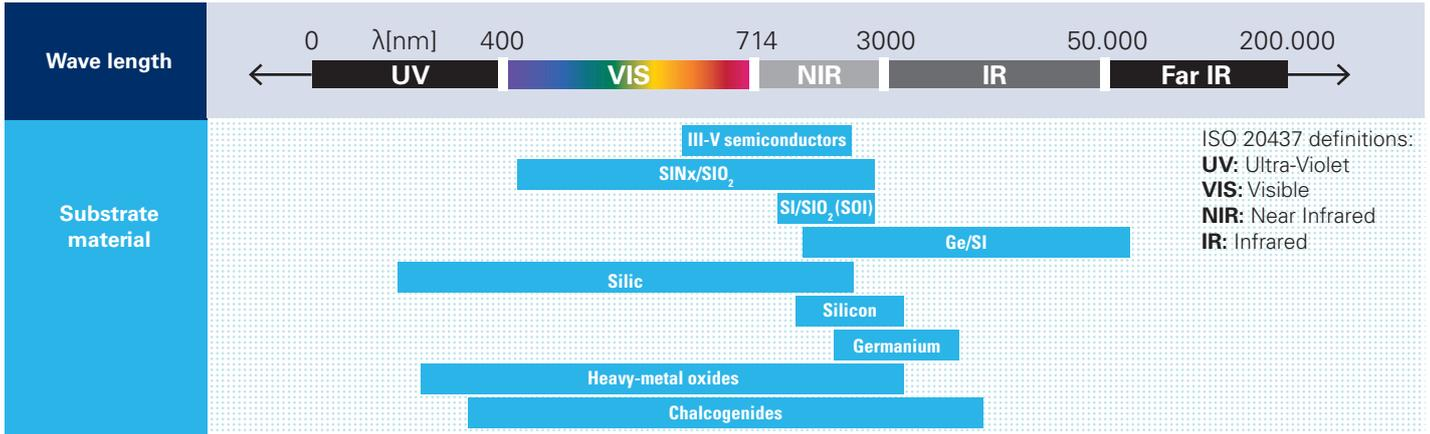
Figure 9 Wavelength of operation of PIC platforms and materials<sup>5)</sup>
