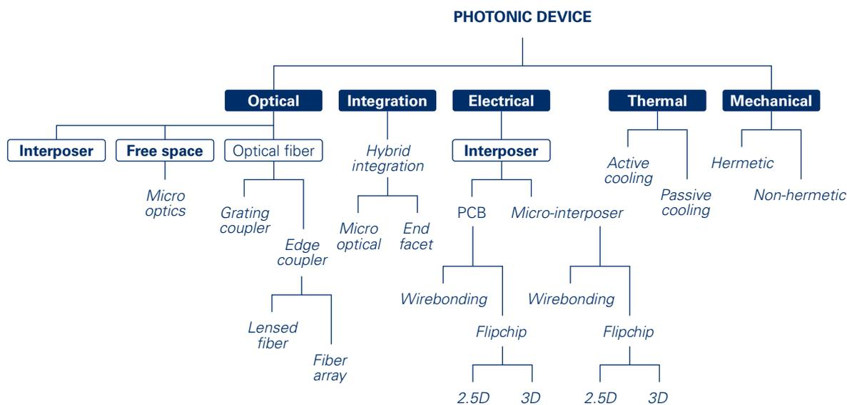
**Figure 11** Organization chart providing a breakdown of the key packaging technologies, including; optical, electrical, thermal and mechanical aspects.<sup>9)</sup>
