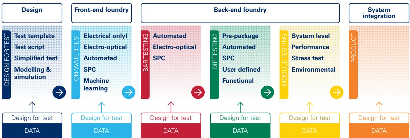
**Figure 15** Test framework for data flow and exchange across production chain from a design to product ([www.openepda.org](http://www.openepda.org))<sup>13)</sup>
