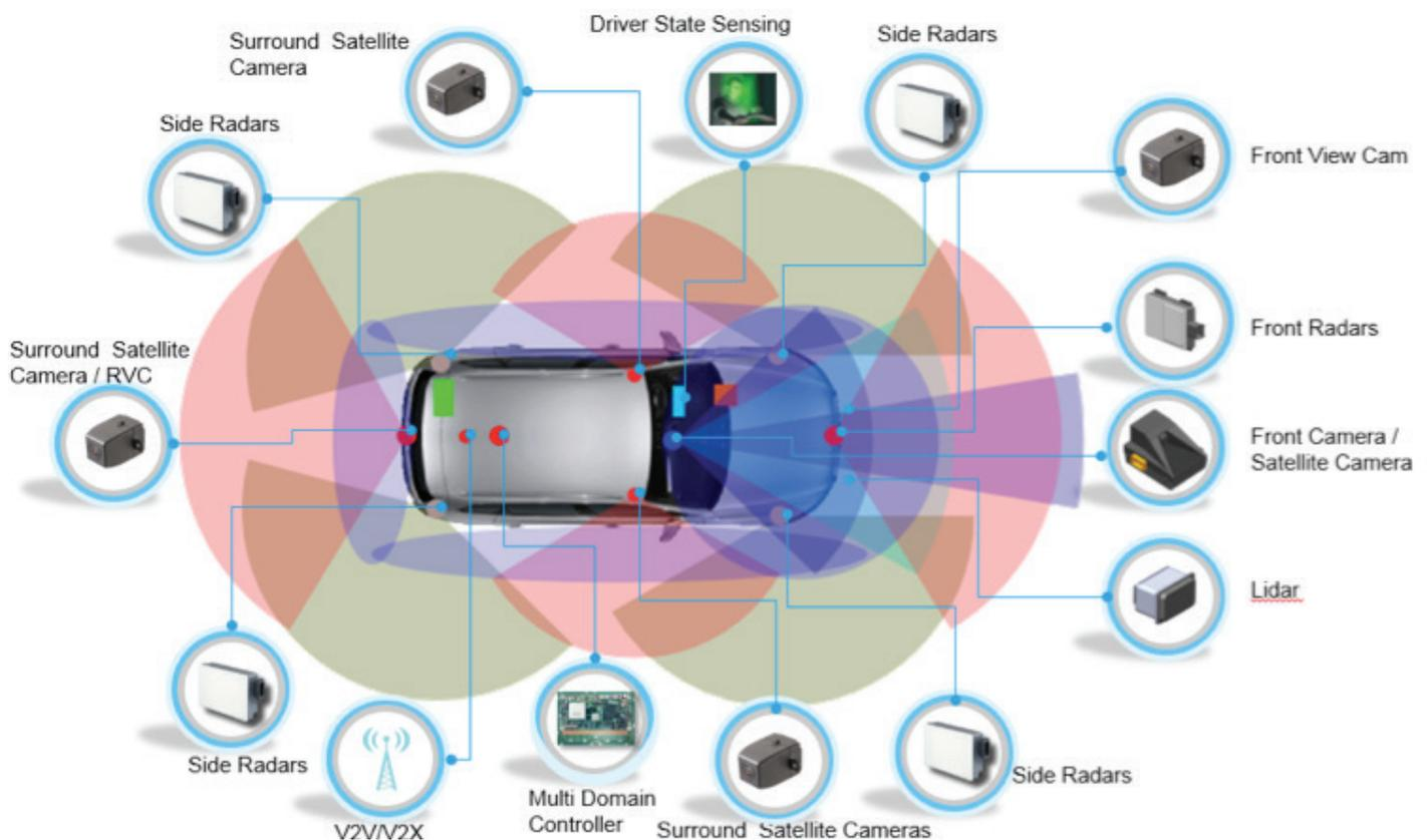
Figure 6 Subset of sensors used for autonomous vehicles
