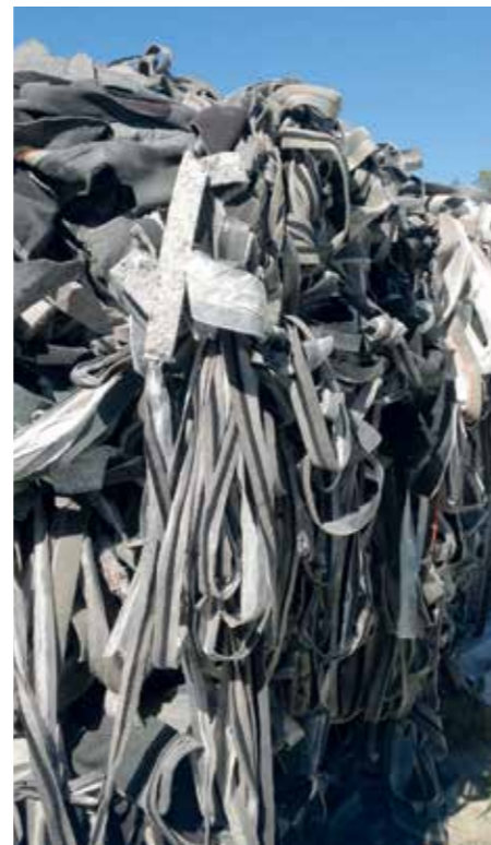
Recycled materials used as fuel in Harleyville Plant. These are out of specification mats for the automotive industry, which, due to their high caloric power, can be used as a replacement for traditional fossil fuels, known as co-processing activity.
