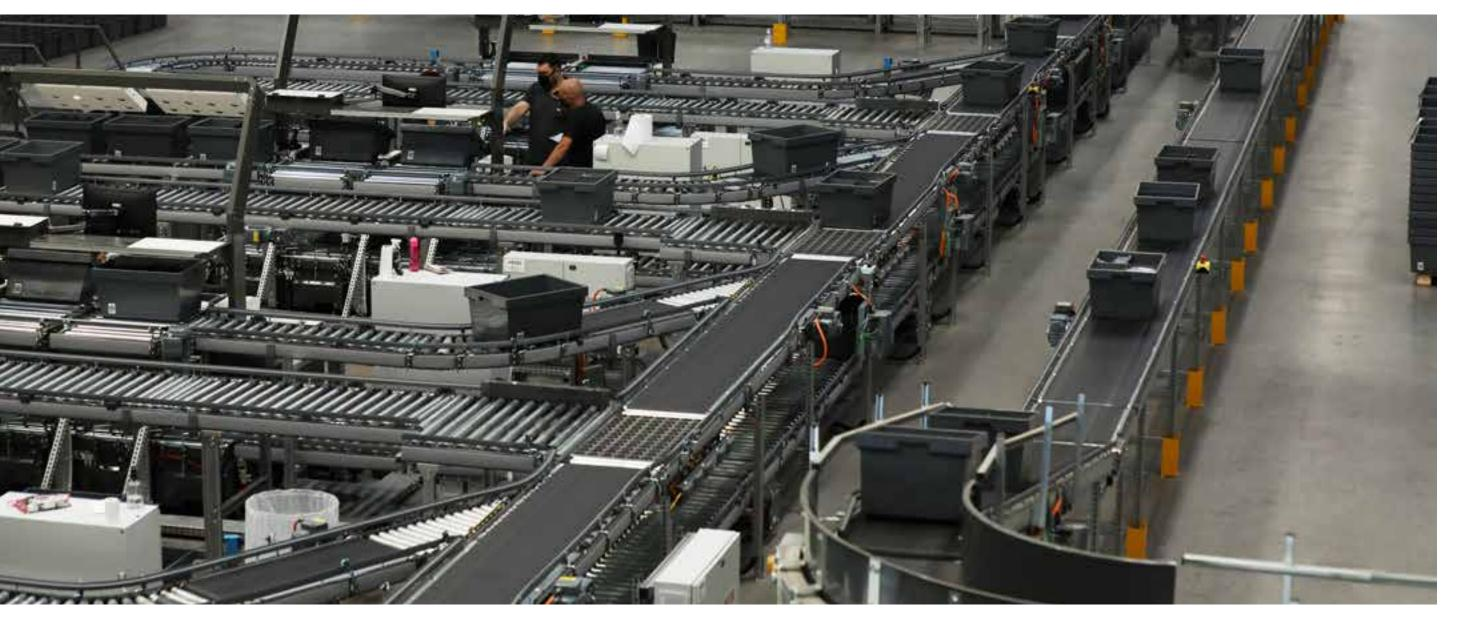
The OSR Shuttle™ automation system allows you to efficiently organize logistics processes, facilitating the storage, separation and sequencing of goods, orders and raw materials in a space-saving manner. Robotization allows an average assembly time per order of around 5 minutes, while the current process took one to two hours. The system is already integrated with the new distribution center management system, ensuring assertive management of tasks and stock.
