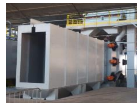
Powder Coating Line (Blasting Process)
