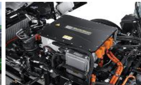
Auxiliary Electrical Control
