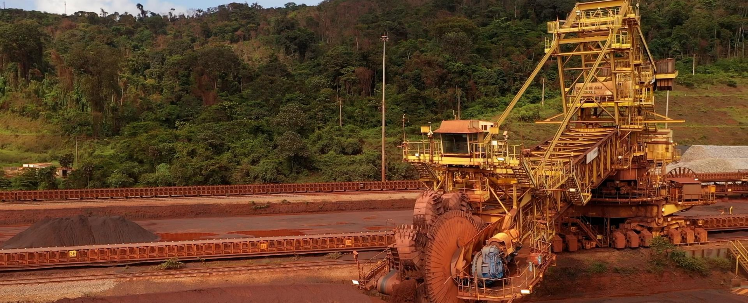
Autonomous stacker reclaimer in Serra Norte stockyard (March 2022)
