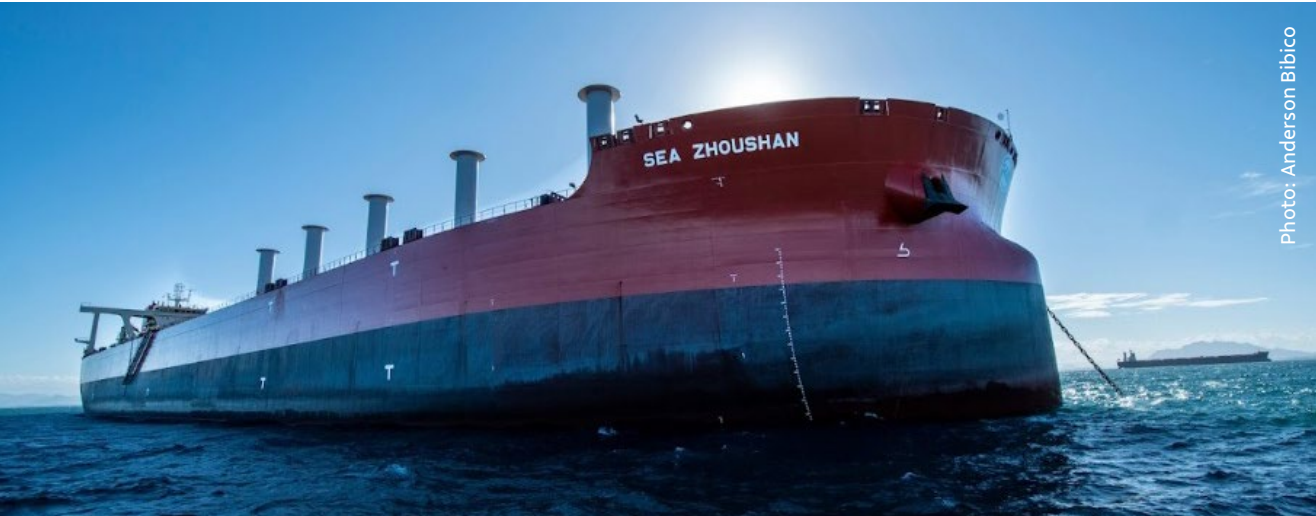
Espírito Santo (ES), Brazil – Port of Tubarão receives the world's first ore carrier equipped with rotor sails. The ship Sea Zhoushan is a Guaibamax
