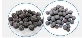
Iron ore fines are agglomerated into pellets and then hardened using a furnace to produce iron ore pellets. These are typically fed into a blast furnace or a direct reduction furnace as part of the steelmaking process.
