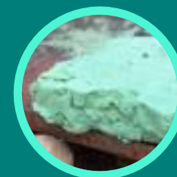
Nickel hydroxide product from water treatment (>20% Ni)
