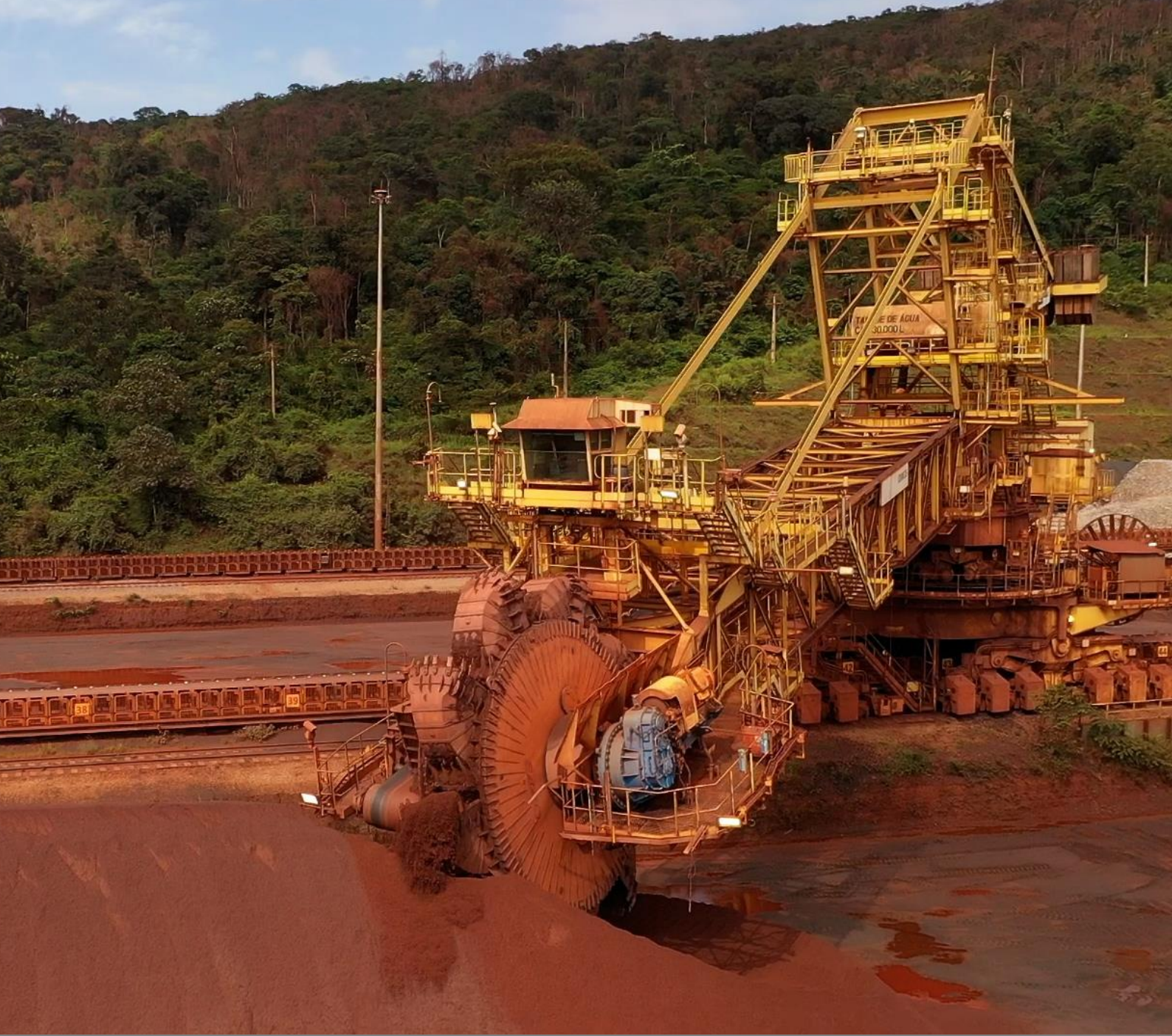
Autonomous stacker reclaimer in Serra Norte stockyard (March 2022)
