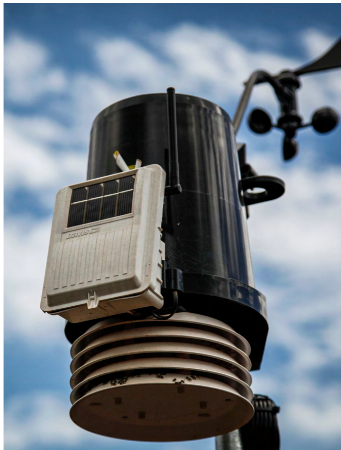
Detail of the meteorological station, which measures temperature and humidity, wind direction and speed, rainfall (rain gauge), and barometric pressure. Photo: Paulo Moreira
