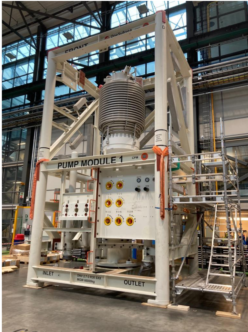
Pumping module (MPP) assembly and testing in Norway
