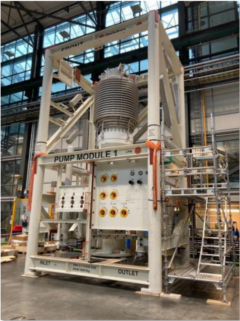
Multiphase pumping module (MPP) completing assembly and testing (Norway)
