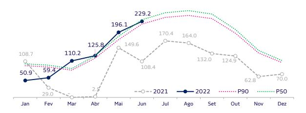
In 2Q22, the generation of Ventos do Araripe III 184 MWavg, 110% above 2Q21 (88 MWavg) and above P50, after the reestablishment of the transformers of the Collecting Substation.
