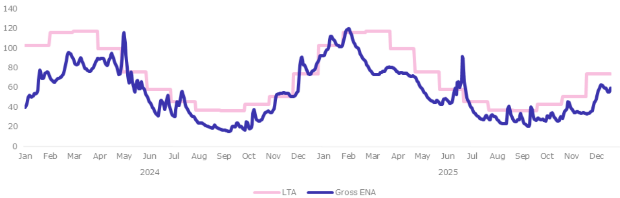
| Chart 1 | Daily Gross Natural Inflow (ENA) in the National Interconnected Grid (SIN) (GWavg)
