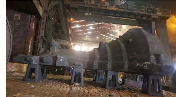
Casting of the turbine housing
