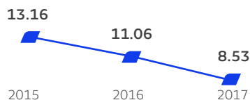
Water consumption in the plant per ton of aluminum produced (m 3 /ton)
