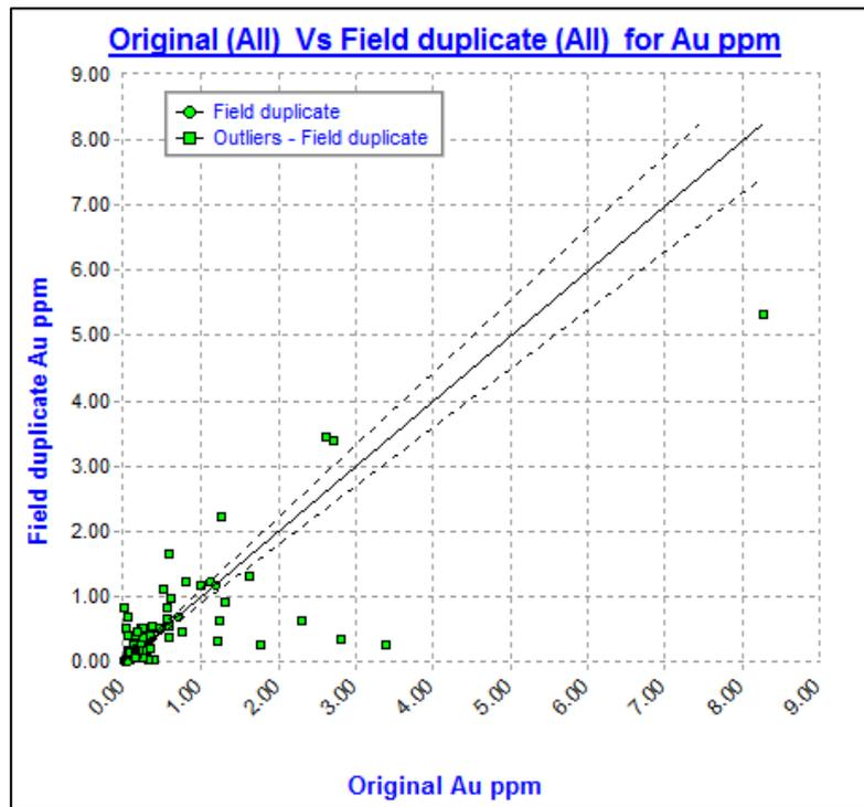
Figure 67: Comparison between original BV assays and re-assay by ALS- Field Duplicates (Crusader, 2012).
