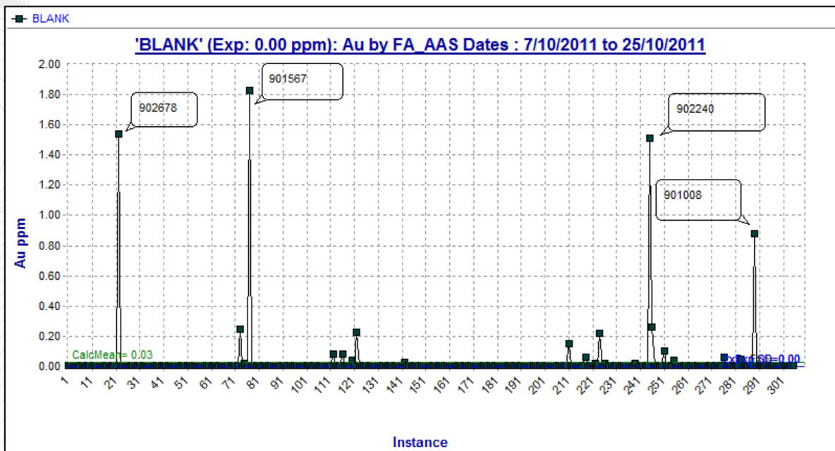
Figure 68: Comparison between original BV assays and re-assay by ALS - Blanks (Crusader, 2012).
