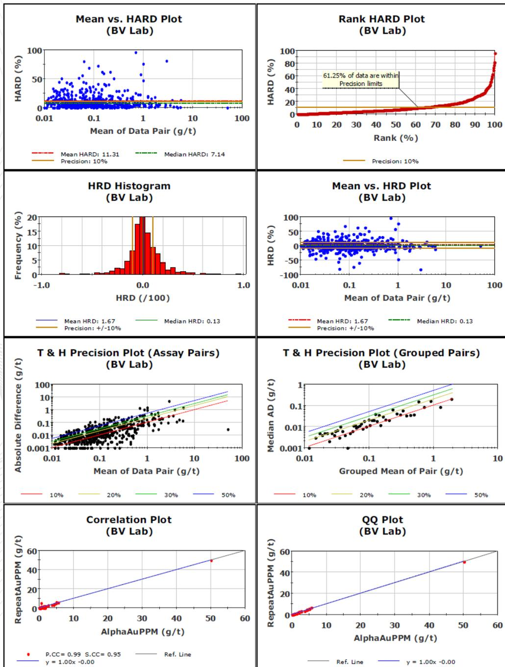
Figure 57: Pulp duplicates performance in BV Lab (Crusader, 2012).
