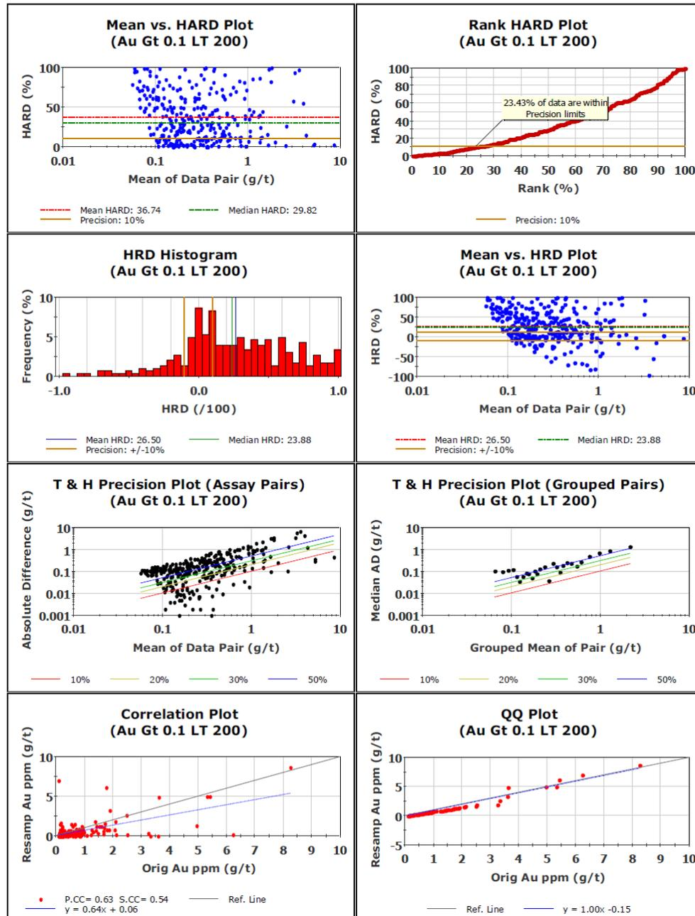
Figure 63: Comparison between original and re-assayed samples in BV lab (Crusader, 2012).
