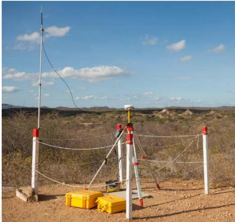
Figure 45: Crusader’s survey base station for differential GPS (2012).
