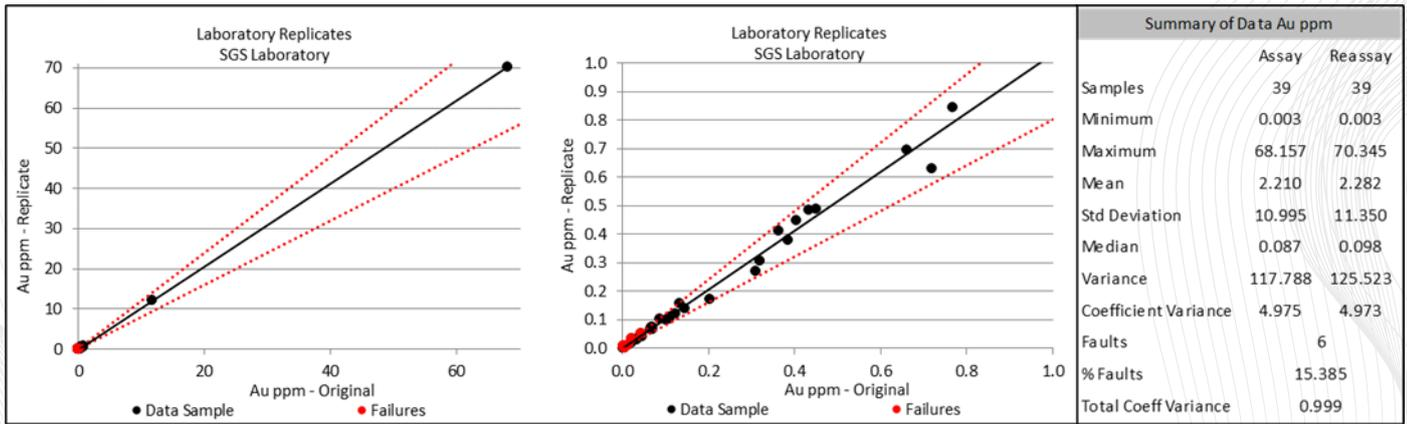
Figure 81: External QA/QC - Lab replicates.
