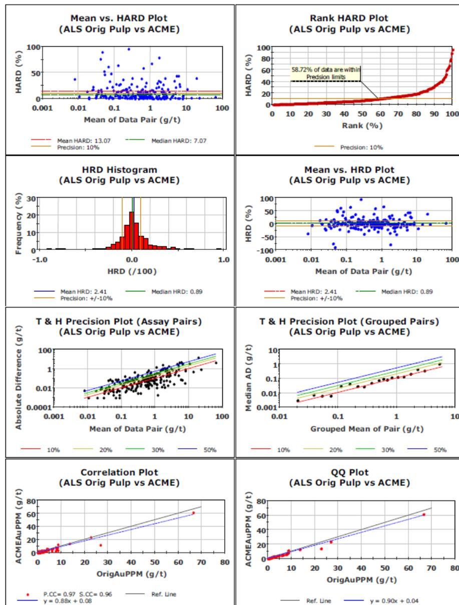
Figure 74: Comparison between ALS Lab assays versus ACME lab-pulps (Crusader, 2012).
