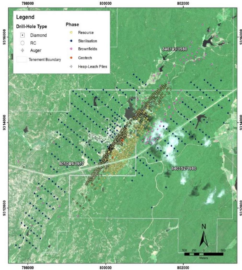
Figure 43: The Crusader's drilling at Borborema Project
