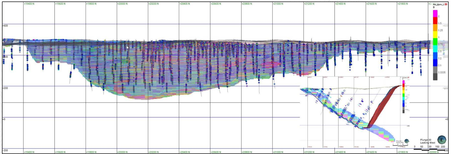
Figure 109: Long section, looking west of the economic pit shell. Insert image shows cross section, looking North (Source: SRK, 2022).
