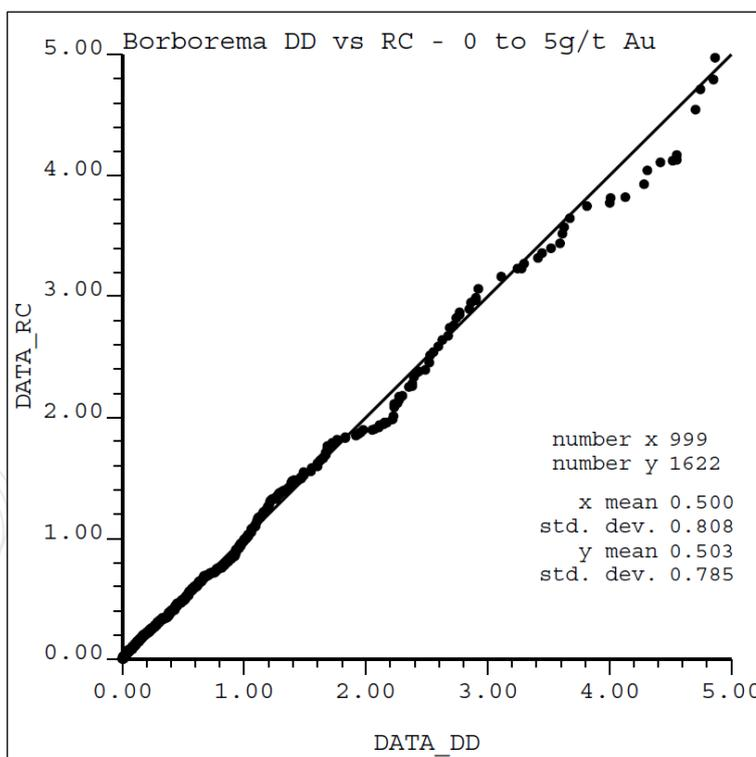
Figure 82: Q-Q plot of RC versus DDH assay less than 5 g/t Au. (Source: Big River data room, 2021).
