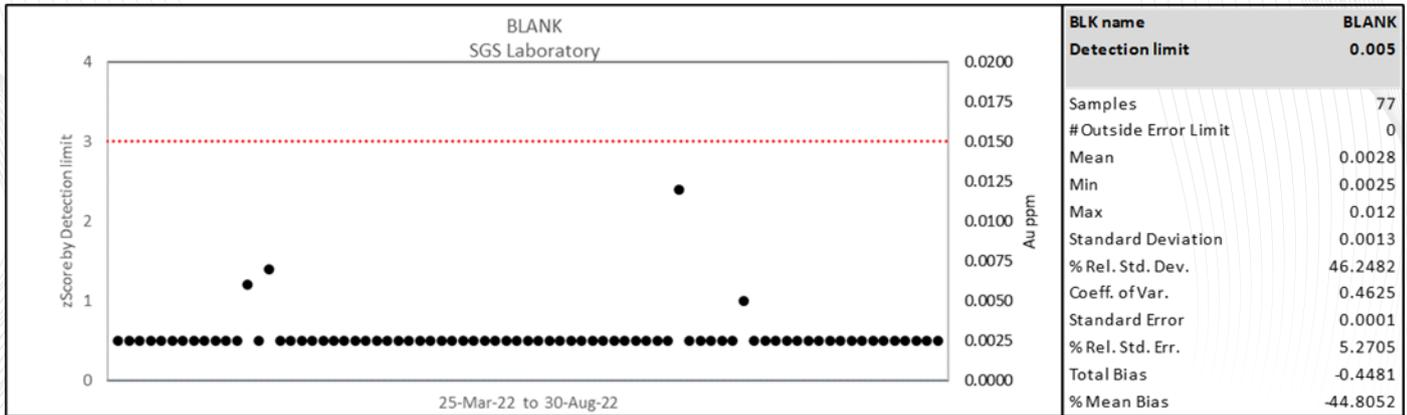
Figure 75: Internal QA/QC- Blank samples.
