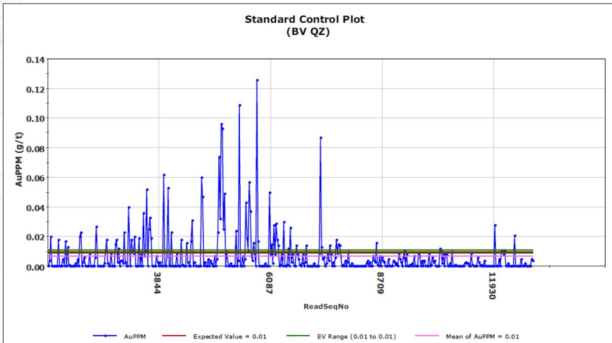
Figure 55: Lab blanks (quartz wash) performance (Crusader, 2012).
