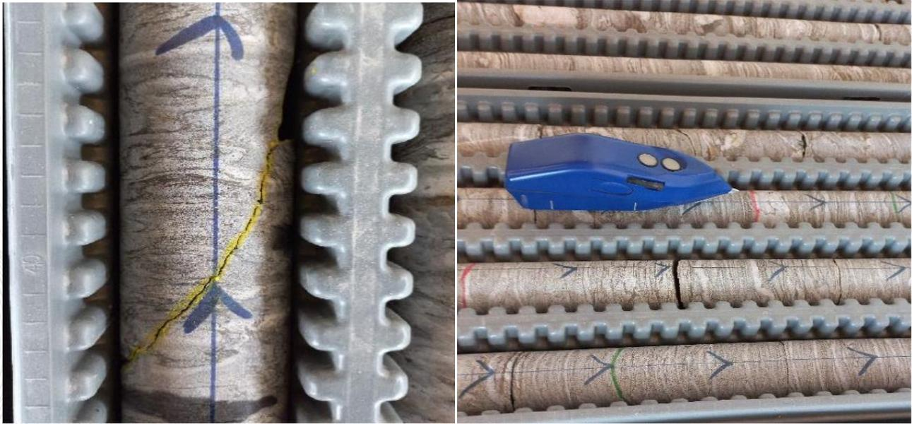
Figure 51: IQ-LOGGER Tool for identifying marked core from oriented drill holes.
