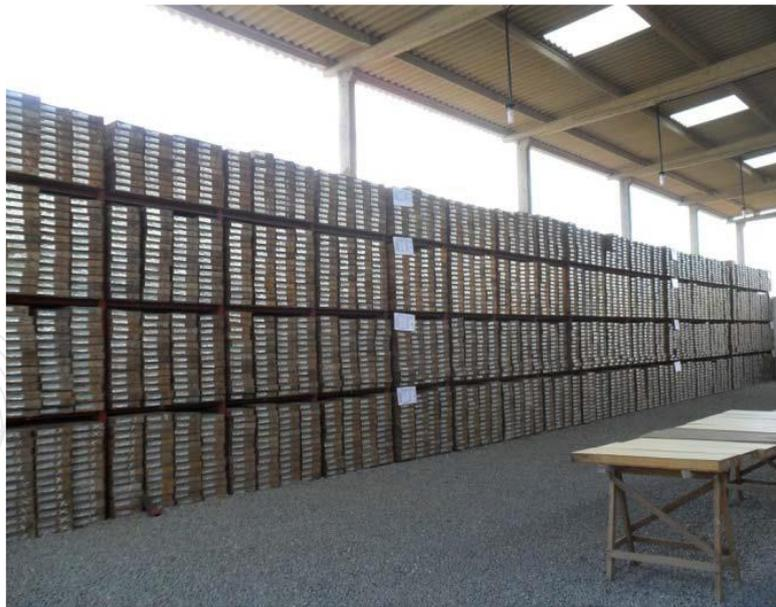
*Figure 50: Borborema core boxes in core shack.*
