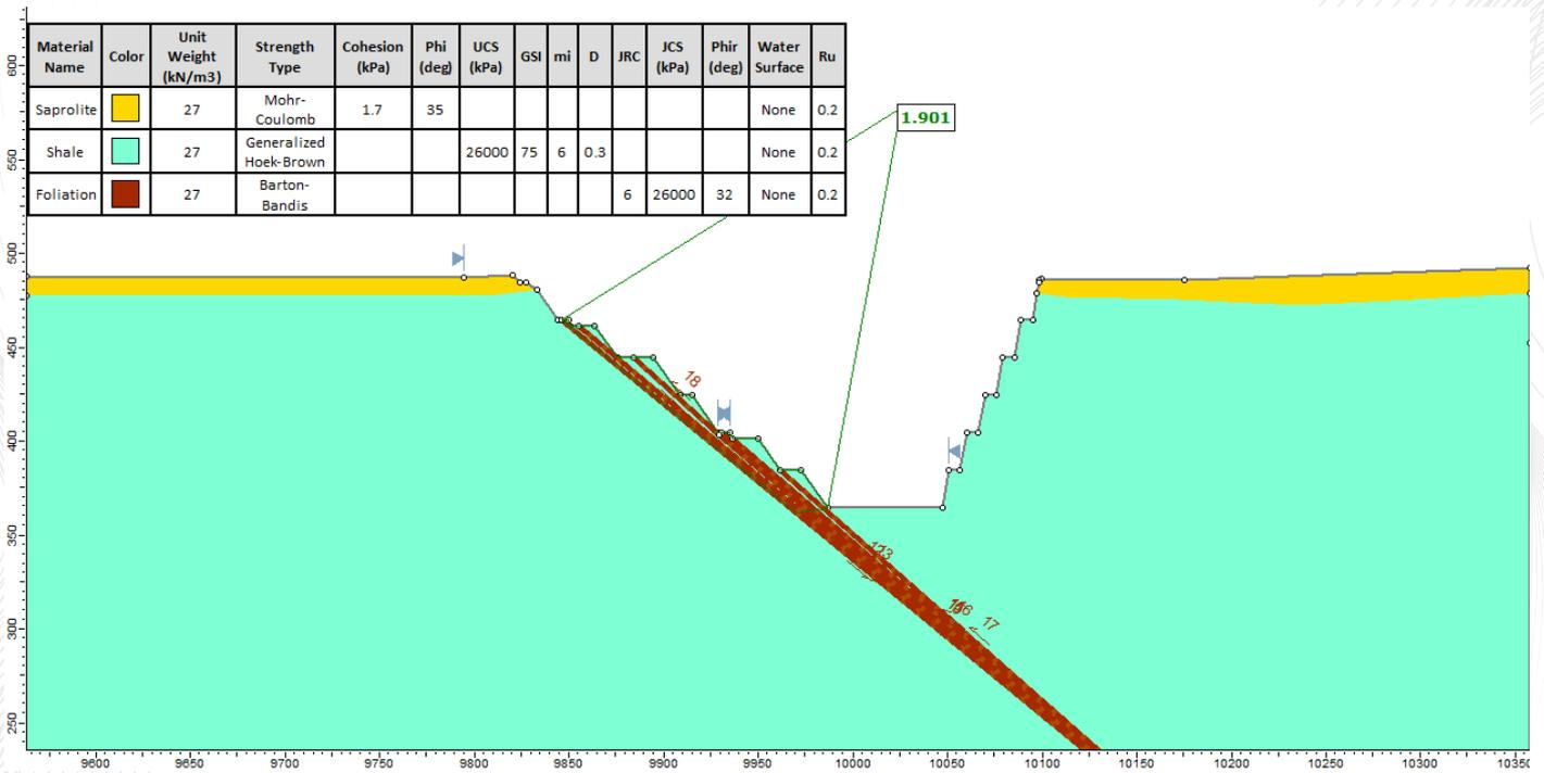
Figure 113: Stability analysis of the western slope – overall.
