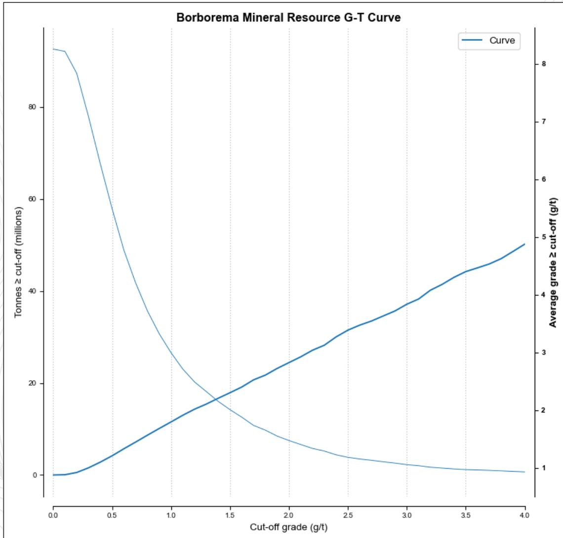
Figure 110: Grade x Tonnage curve.
