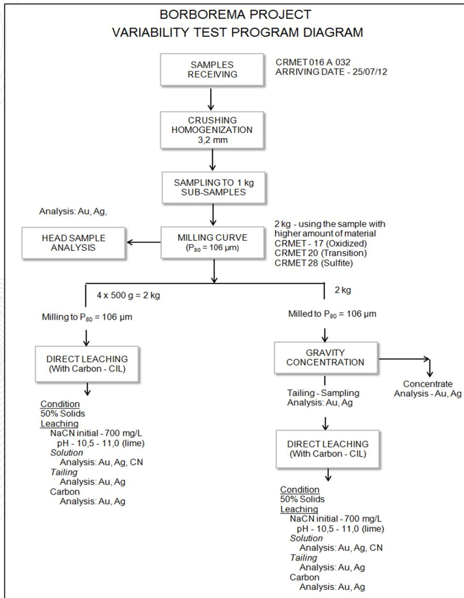
Figure 86: Leach Test Procedures - Variability Testing.
