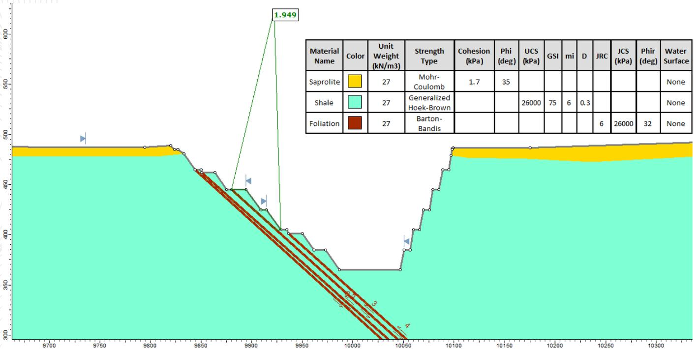
Figure 114: Stability analysis of the western slope - inter-ramp.
