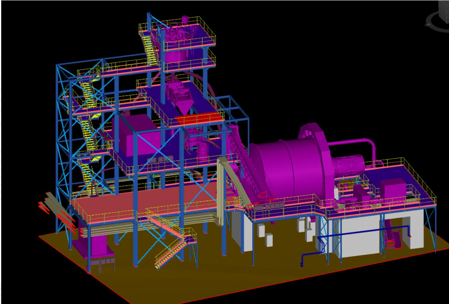
Figure 121: Grinding area schematic view.
