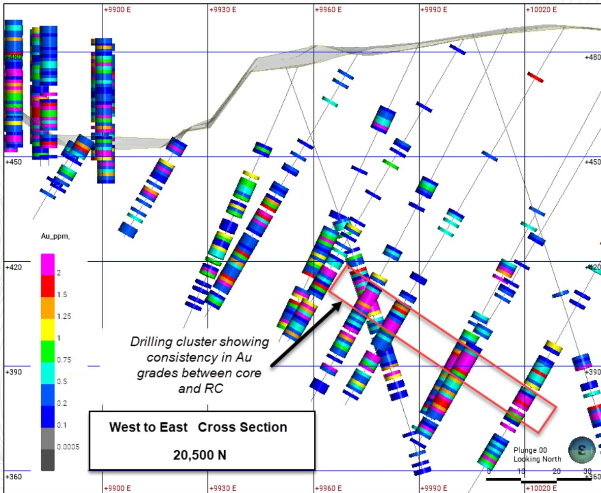
Figure 83: North-looking vertical cross section showing RC and DDH holes coloured by Au grade. (Source: SRK, 2021).
