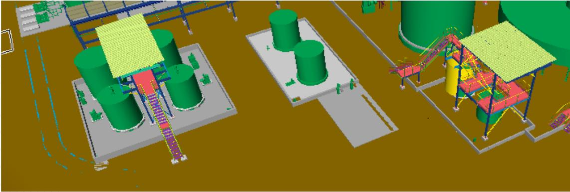
Figure 126: View of the reagent area - From right to left: hydrated lime, hydrochloric acid, caustic soda, sodium metabisulfite, and copper sulphate.
