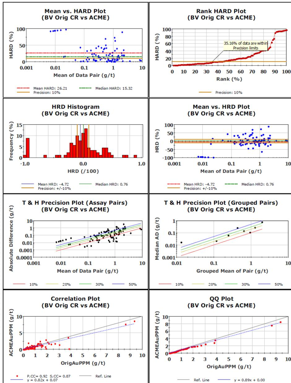
Figure 73: Comparison between original BV assays versus ACME Lab-Coarse Rejects (Crusader, 2012).
