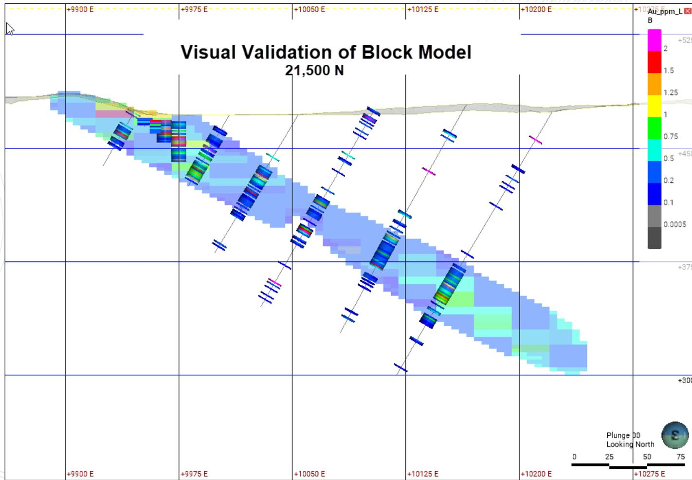
Figure 105: Vertical cross section looking north showing blocks and drilling coloured by Gold Values (ppm Au).
