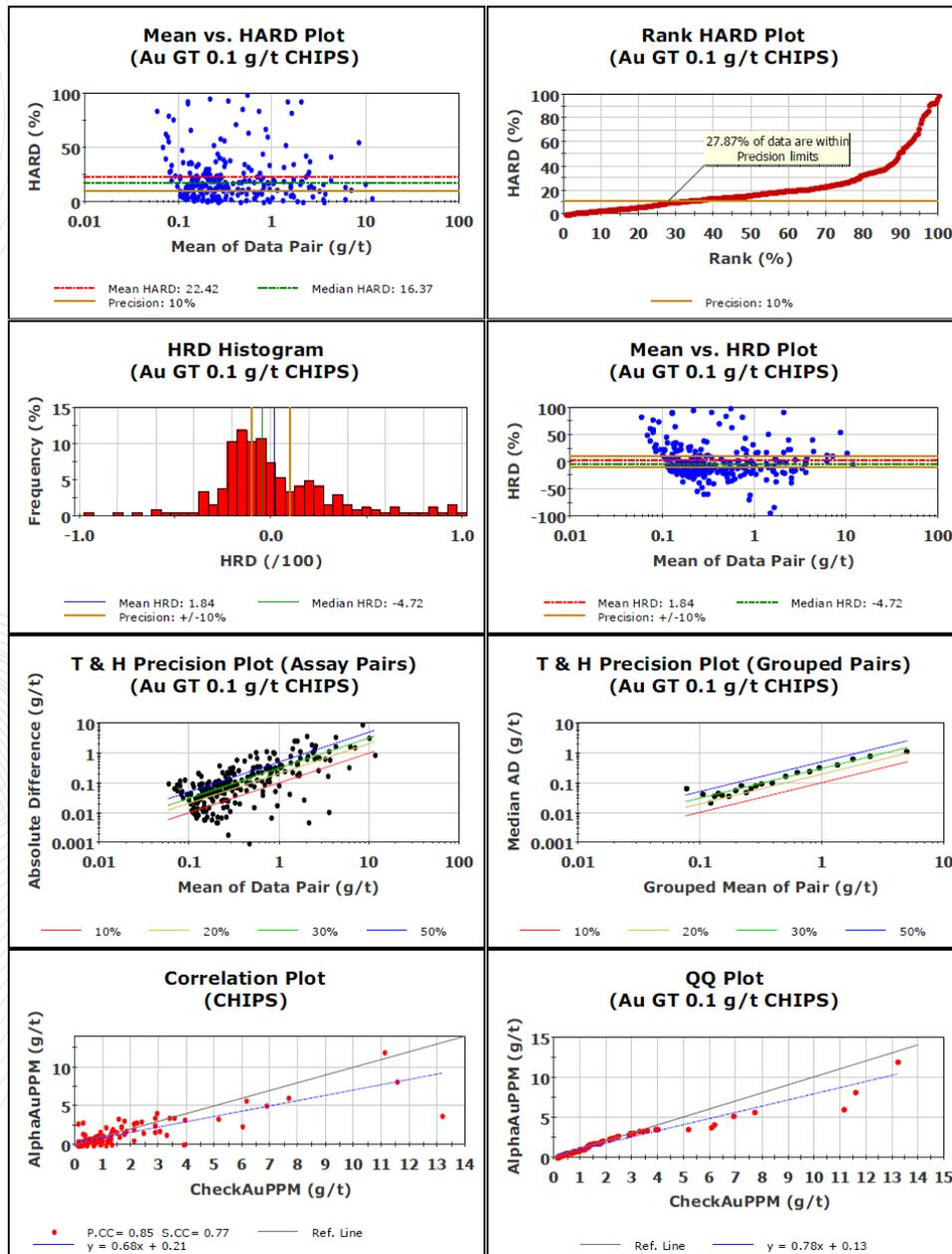
Figure 71: Comparison between original BV assays and re-assay by Ultratrace (Crusader, 2012).
