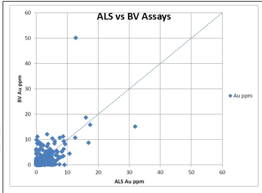
Figure 65: Comparison between original BV assays and re-assay by ALS - all data (Crusader, 2012).
