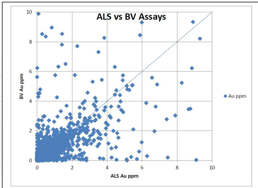
Figure 66: Comparison between original BV assays and re-assay by ALS - Au < 10g/t (Crusader, 2012).
