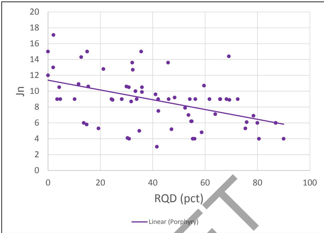
Figure 4-7. Drill Hole Comparison Between Logged RQD and Barton Jn Parameter for Porphyry Domain.
