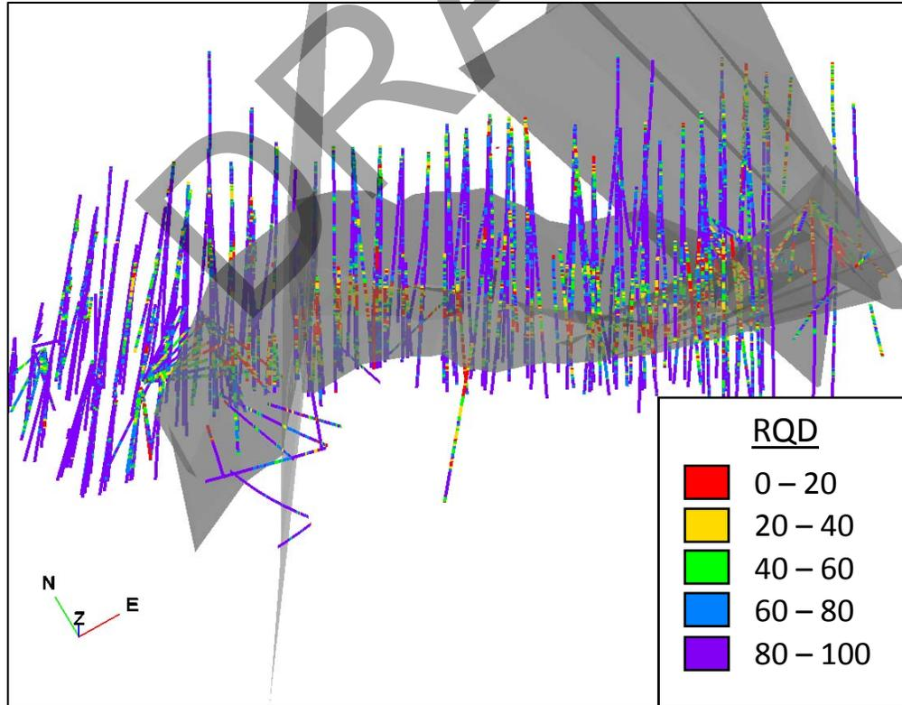
Figure 4-16. Oblique View (Looking Northeast) of Fault Domain Wireframes (Grey) and Low RQD Composite Intervals (RED).
