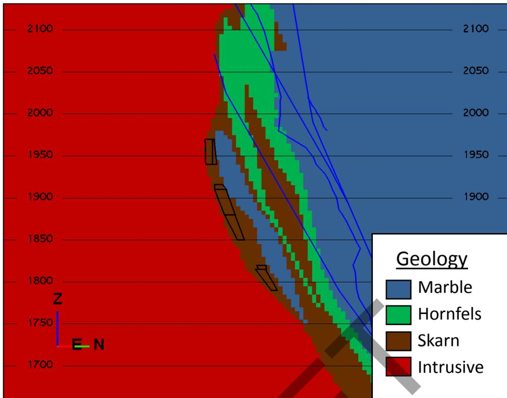
Figure 3-3. Cross Section (42) Presenting Interpreted Geology Boundaries, Fault Traces (Blue), and 10 Meter Slope Shapes (Black) (Looking Northwest).
