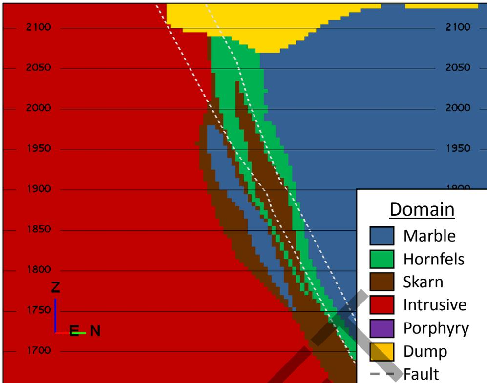
Figure 4-13. Cross Section (42) Presenting Geotechnical Domain Boundaries, Fault Domain Boundary Sub-divides All Block Model Domains.
