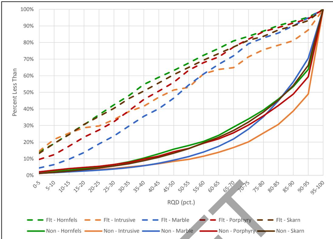
Figure 4-11. Cumulative Distribution of Drill Hole Composite RQD by Geotechnical Domain
