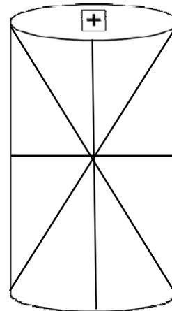
**NOTES:** Heavy sulfides. Testing surfaces capped and voids filled with hydrostone to keep sample intact. Resid Load: 35,000 lbs
