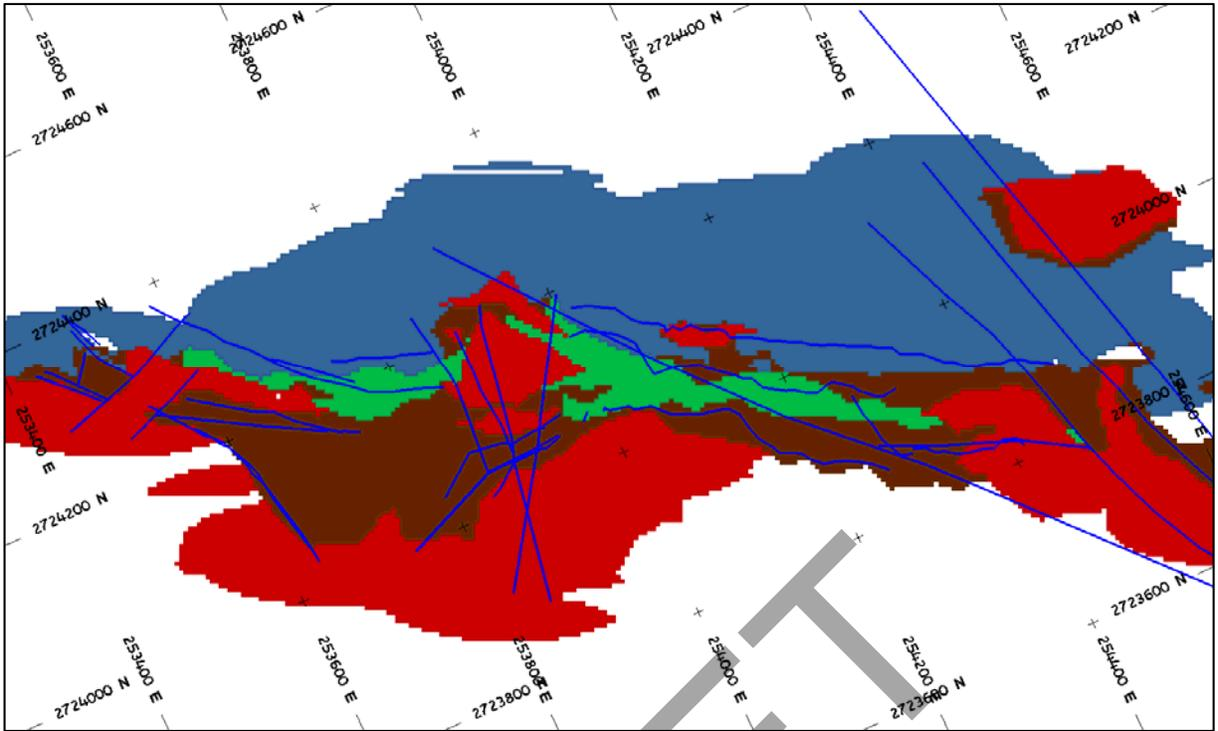
Figure 3-5. Fault Traces (Blue) in Plan View (2040 L) Showing Cross Cutting Relationships of Transverse and Bedding Parallel Faults
