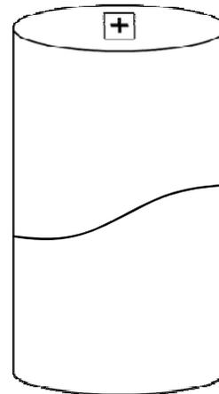
**NOTES:** Heavy sulfides. Testing surfaces capped and voids filled with hydrostone.
