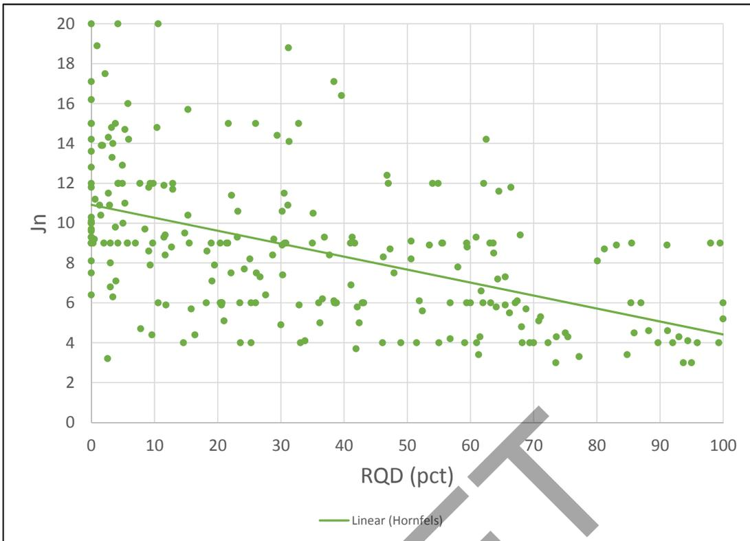
Figure 4-5. Drill Hole Comparison Between Logged RQD and Barton Jn Parameter for Hornfels Domain.
