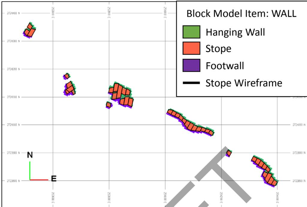
Figure 4-33. Plan View of 1905 Level Showing Stope Wireframes and WALL Model Codes
