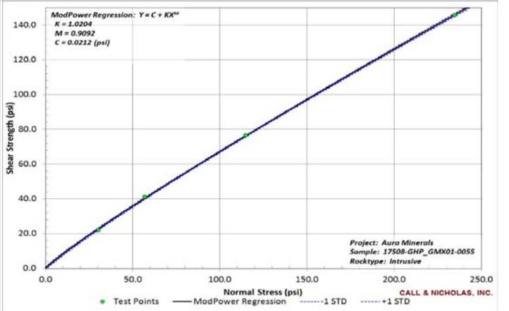
Notes : JRC = 4-8. Well mated and well locked. Sample surface filling is a trace of white, soft, moderately-attached powder.
