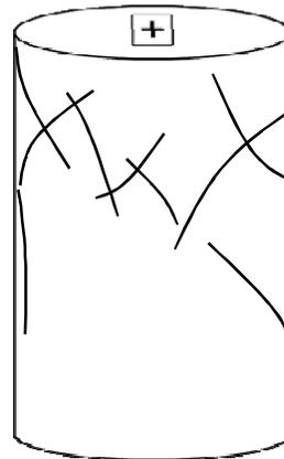
**NOTES:** Sandstone. Heavy Sulfides. Small voids and gouges.
