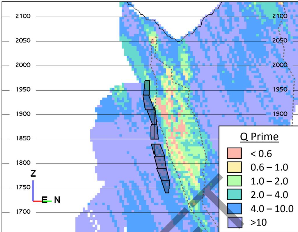
Figure 4-29. Cross Section (24) Presenting Estimated Q Prime with Fault Boundaries (Dashed) and 10 Meter Slope Design (Black).
