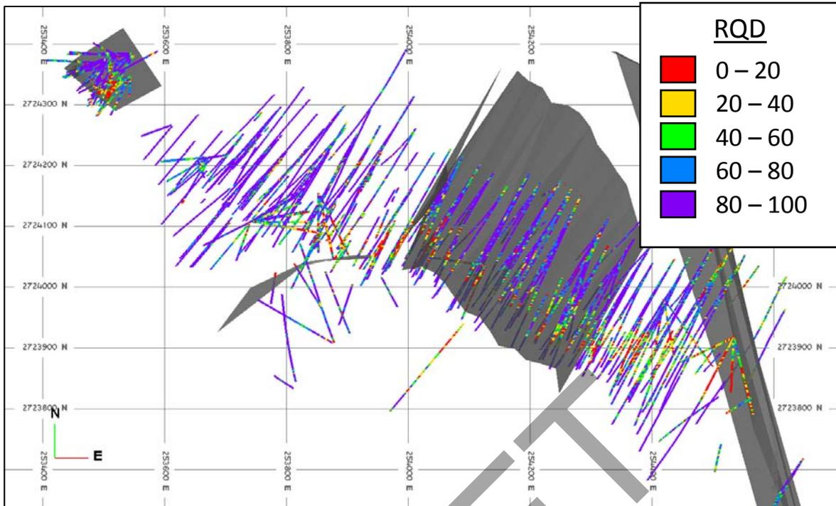
Figure 4-15. Oblique View (Plan View) of Aranzazu Modeled Faults (Grey) and Low RQD Composite Intervals (RED).
