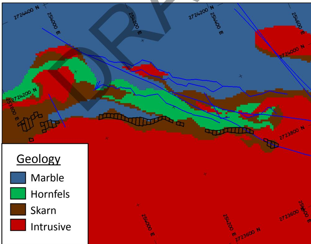
Figure 3-4. Plan View (1875L) Presenting Interpreted Geology Boundaries, Fault Traces (Blue), and 10 Meter Slope Shapes (Black).
