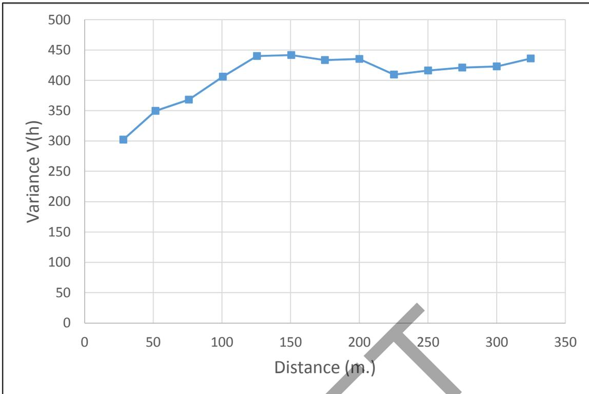
Figure 4-17. Experimental Isotropic Variogram of Marble Domain.
