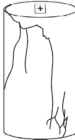
**NOTES:** Heavy sulfides. Sample does not meet end tolerances for flatness.
