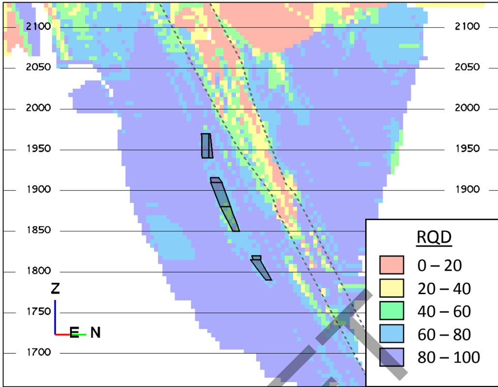
Figure 4-27. Cross Section (42) Presenting Estimated RQD with Fault Boundaries (Dashed) and 10 Meter Slope Design (Black).
