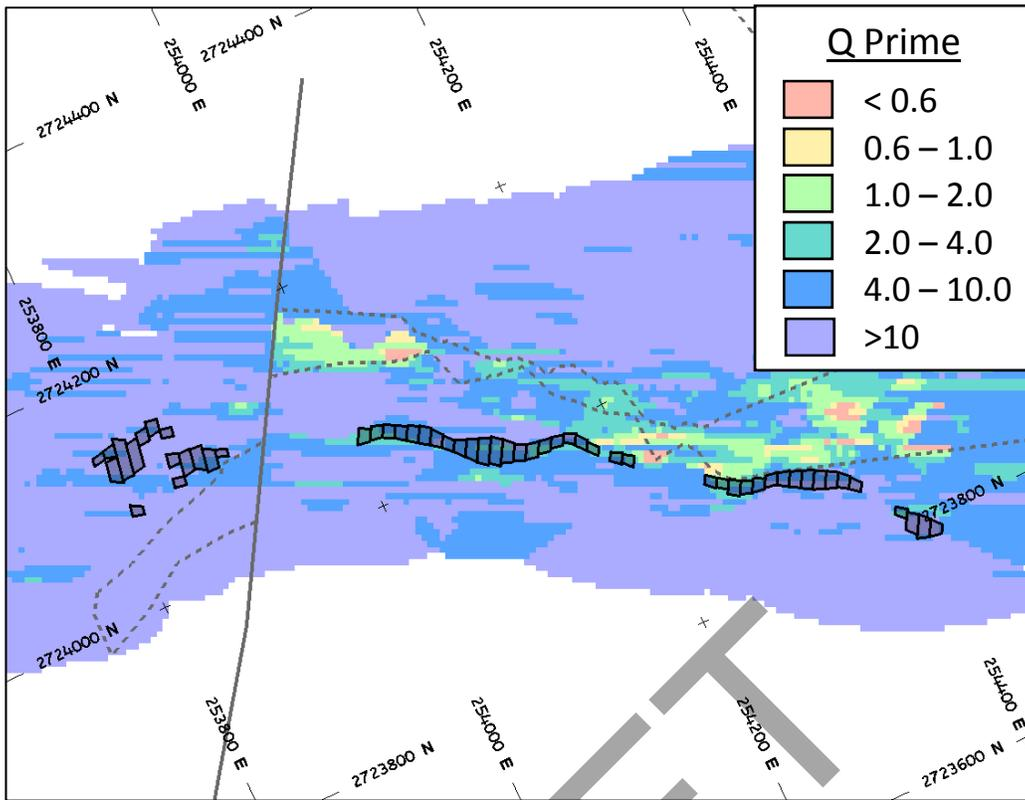
Figure 4-31. Plan View (1875 L) Presenting Estimated Q Prime with Fault Boundaries (Dashed) and 10 Meter Slope Design (Black).
