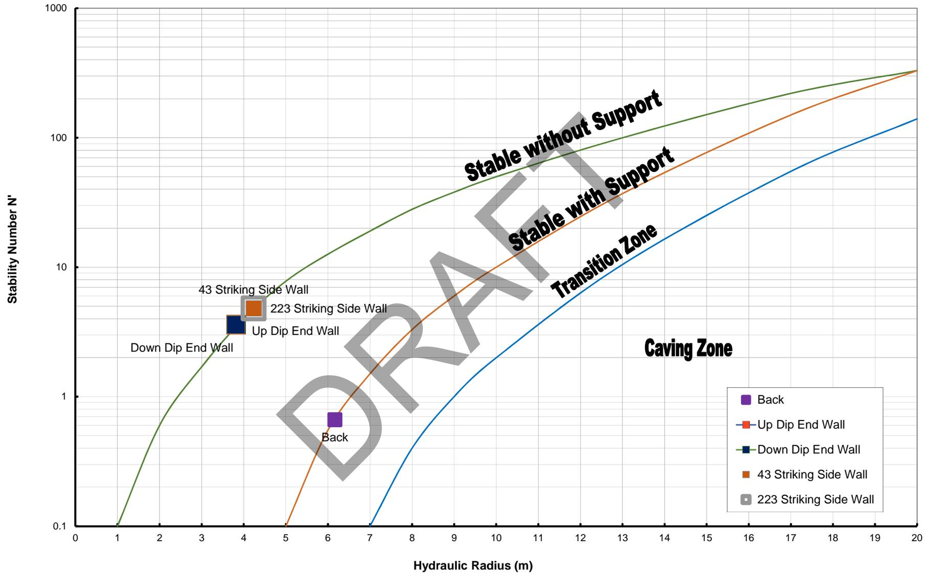
Figure 8-4B. Stability Graph Results for GMT 4 ( $Q' = 2.0$ ); Transverse Mining
