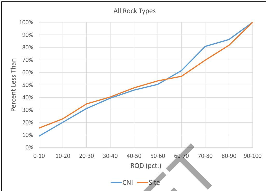
Figure 4-1. Cumulative Distribution of Drill Hole Composite Comparing CNI and Site Logged RQD Data.
