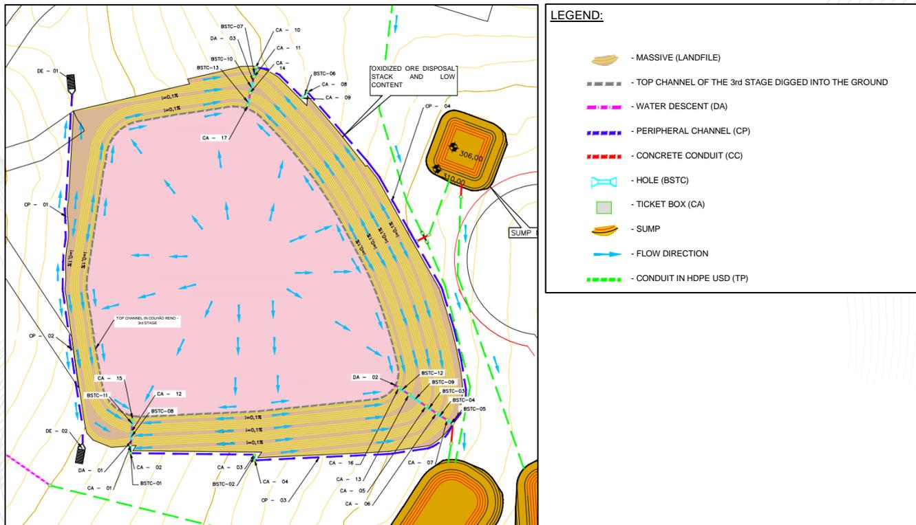
Figure 18-20 - Plant surface drainage Low Grade Ore stockpile - PMBT (GHT, 2022)
