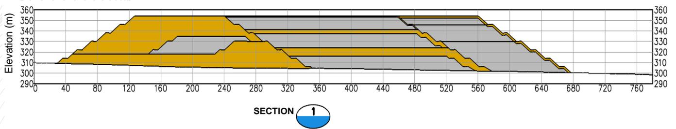
Figure 18-10 - Section slope stability for the PDE stockpiles (MTP-B-DS-5010-GHT-G-0013 - GHT, 2022)
