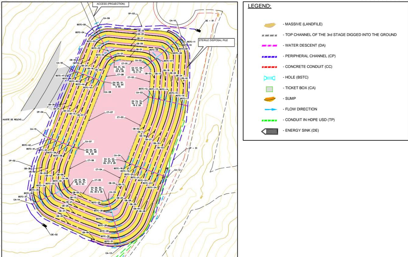
Figure 18-18 – Plant Surface drainage sterile stockpile - PDE (GHT, 2022)
