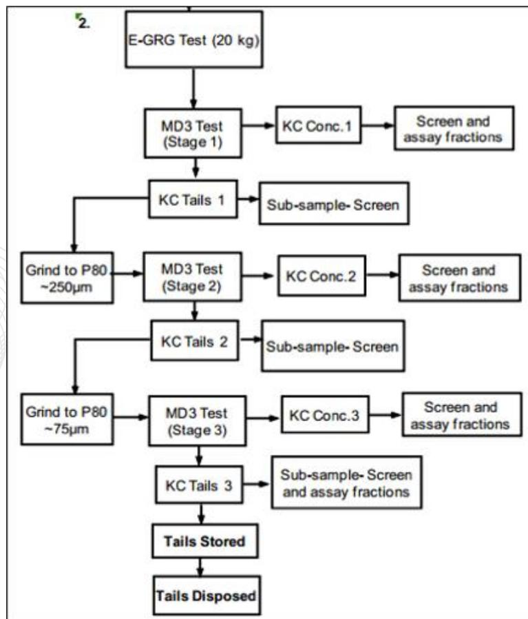
Figure 13-5 - Gravity Recoverable Gold Test Flow Sheet.
