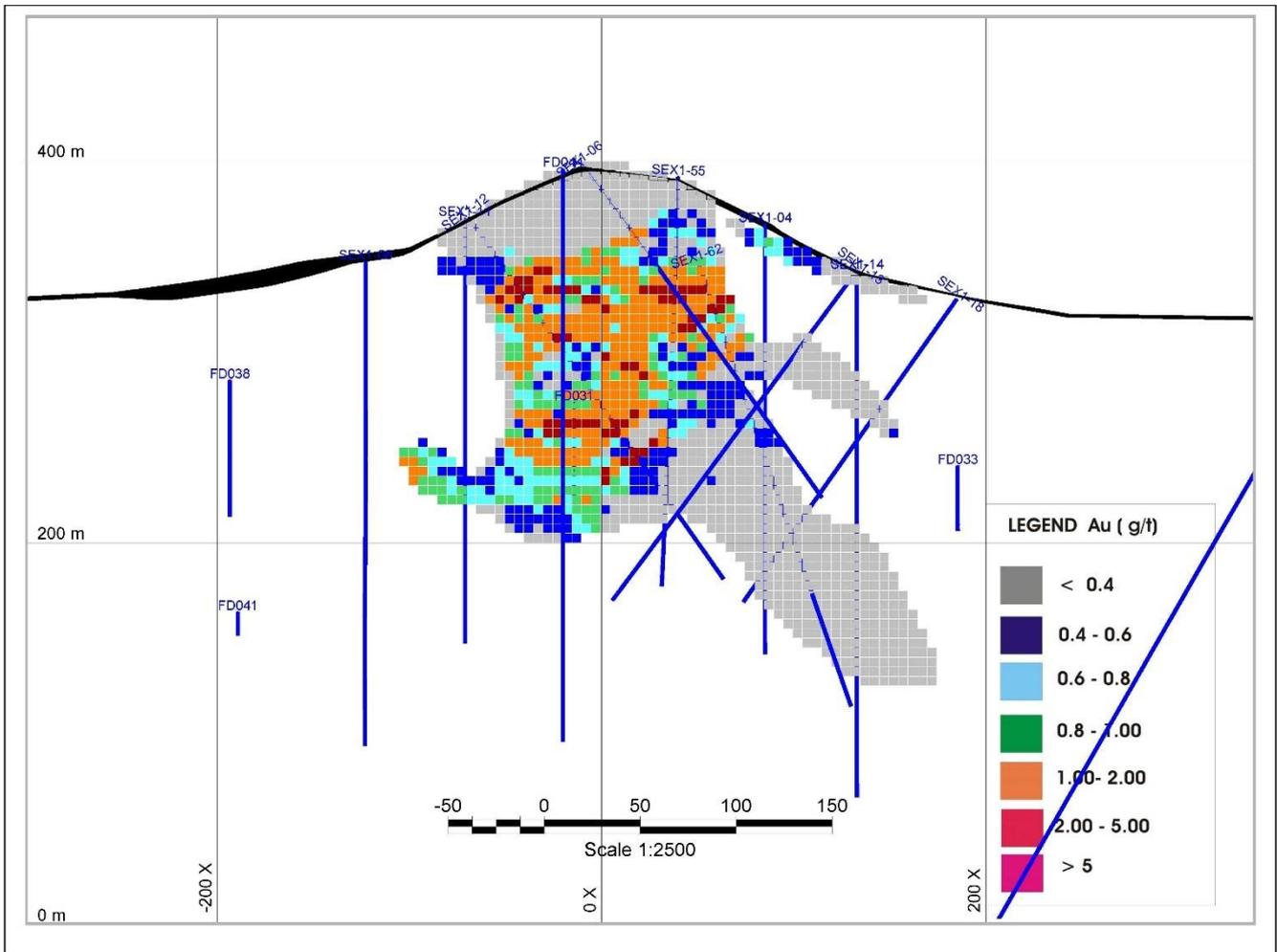
Figure 14-23 - Typical Cross-Section Through the X1 Block Model Estimated Grades (Au) (Looking N).
