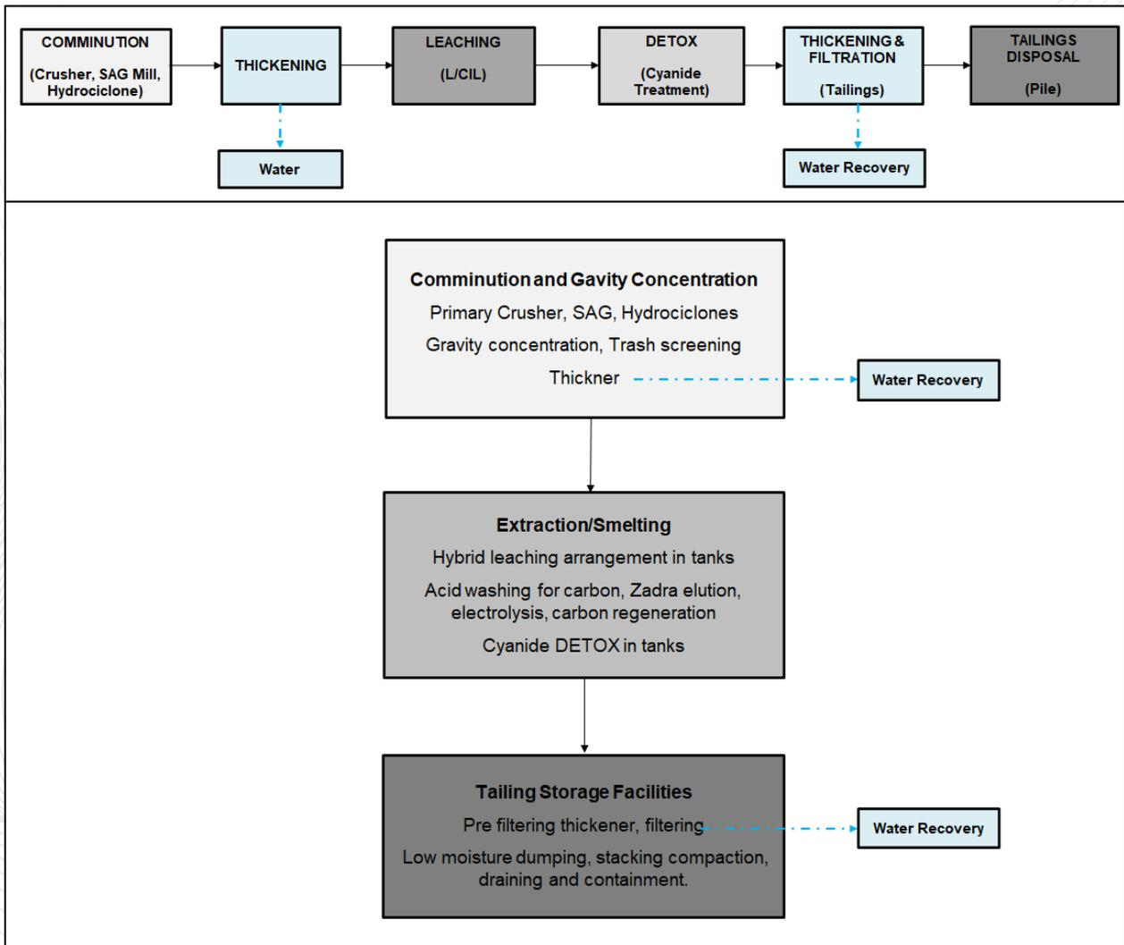
Figure 17-1 - Overall Process Flow Sheet - Matupá Project.
