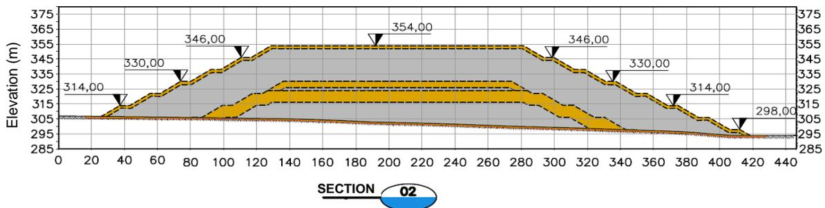
Figure 18-12 - Section 02 slope stability for the PMBT stockpiles (MTP-B-DS-5010-GHT-G-0013 - GHT, 2022)
