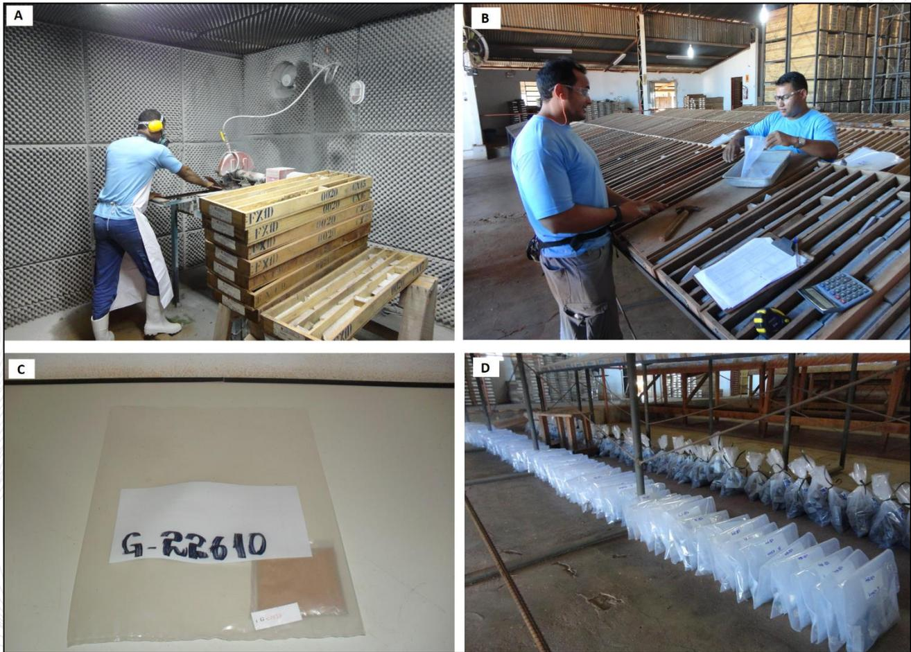
A) Core cutting facility in Rio Novo core-shack; B) Diamond drill core sampling at core-shack; C) Insertion of control samples; D) Samples inserted in tagged plastic bags.
