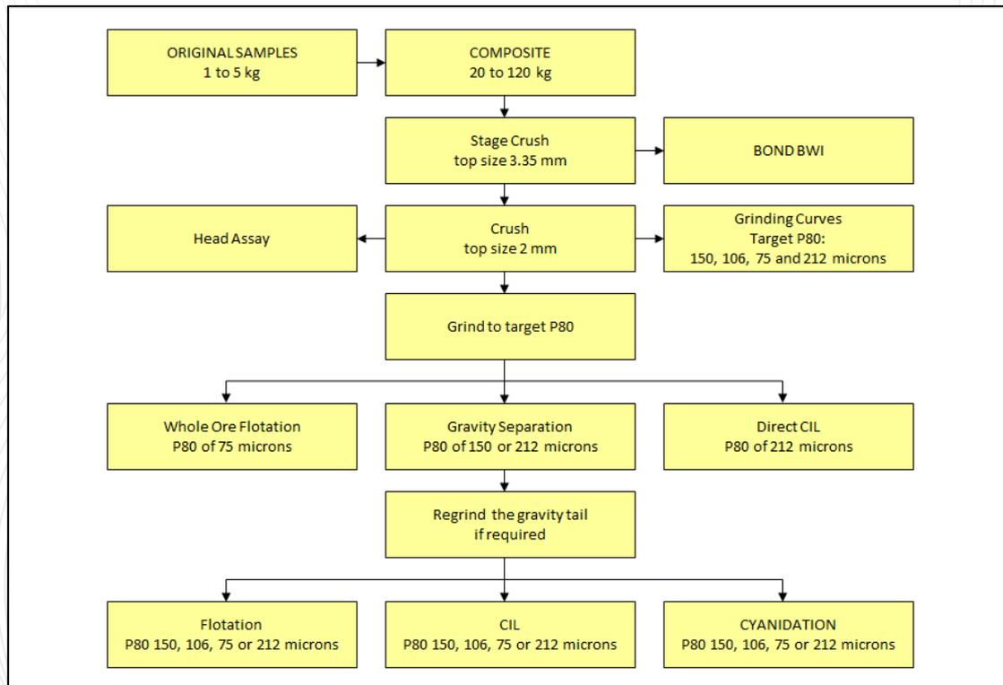
Figure 13-2 - Sample and Test Preparation Flow Sheet Adopted for the First Metallurgical Campaign.
