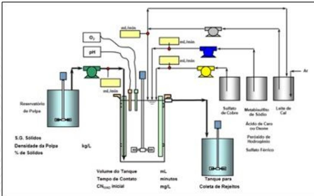
Figure 13-13 - Schematic Diagram of the Process Route Adopted for the Continuous Detox Tests.
