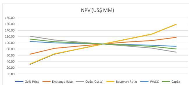
Figure 1-8 - Sensitivity Analysis Graph – NPV.
