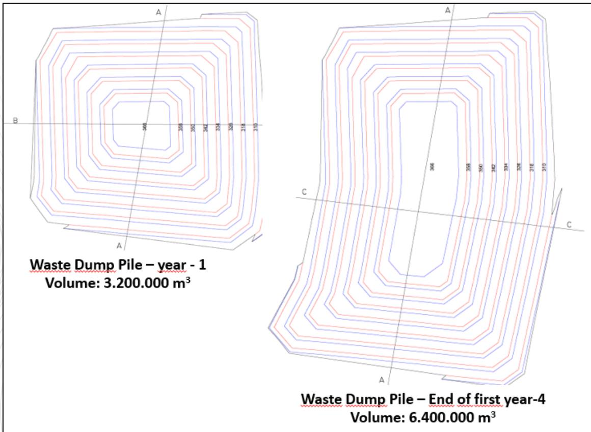
Figure 15-21 - Waste Dump Pile, intermediate dumping phase related to operations year one and year four.
