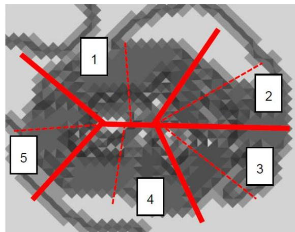
Figure 15-2 - Sectors Defined in X1 Typical Pit and the Sections for the Stability Analysis.
