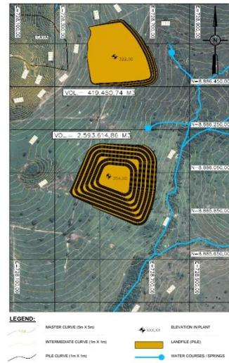
Figure 18-5 – Pre-operation and first year of operation (MTP-B-DS-5010-GHT-G-0003, GHT, 2022)
