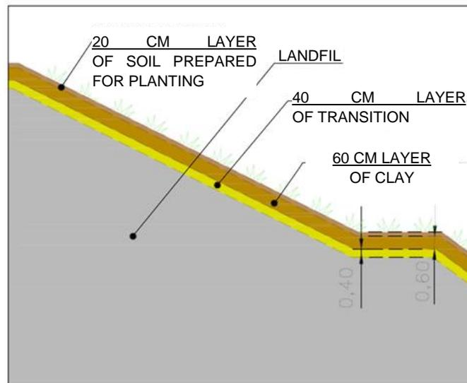
Figure 18-8 – Typical section with transition layer overlaid by clay with low degree, permeability and planting grasses
