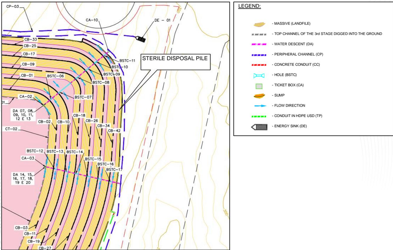
Figure 18-19 – Detail Surface drainage sterile stockpile - PDE (GHT, 2022)
