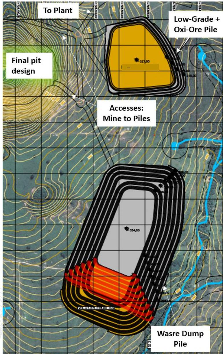
Figure 15-10 - Details of the Final Designed Plans for: Waste Dump Piles, Oxidized Ore and Low-Grade Ore Pile, and Mine Pit Design.
