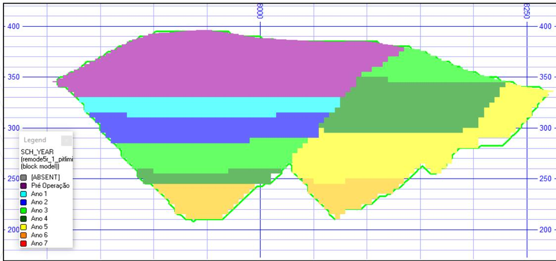
Figure 15-7 - A-A Profile Longitudinal View from Open Pit Design (Figure15-5).
