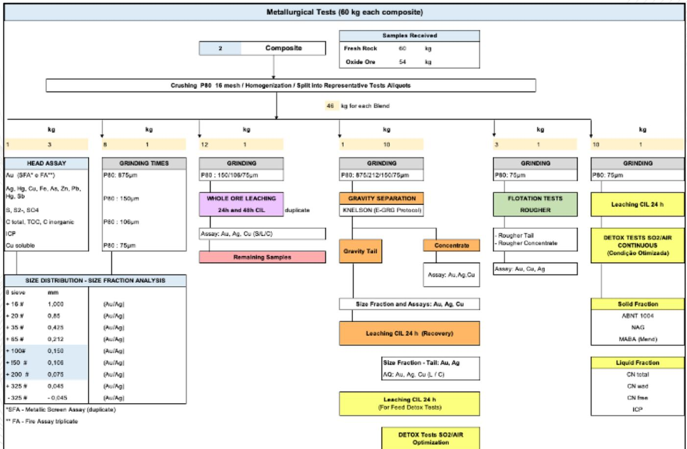
Figure 13-3 – Sample Preparation and Testing for the Second Campaign.
