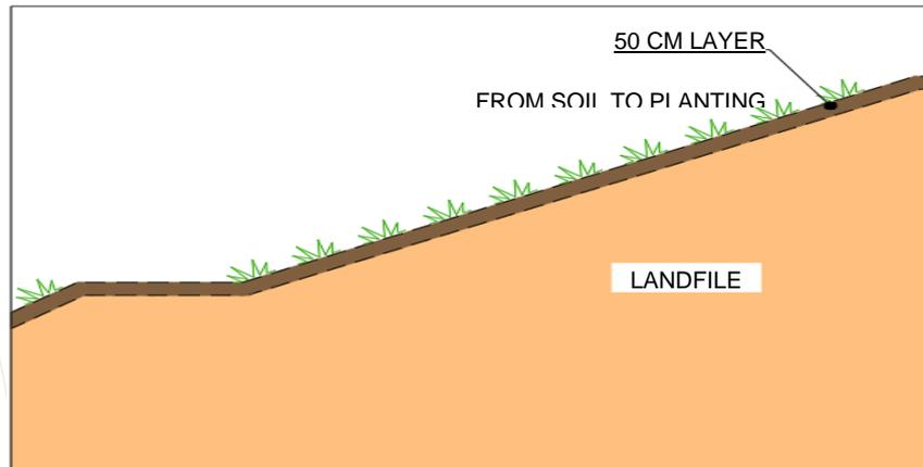
Figure 18-16 – Typical section waste stockpile (GHT, 2022)
