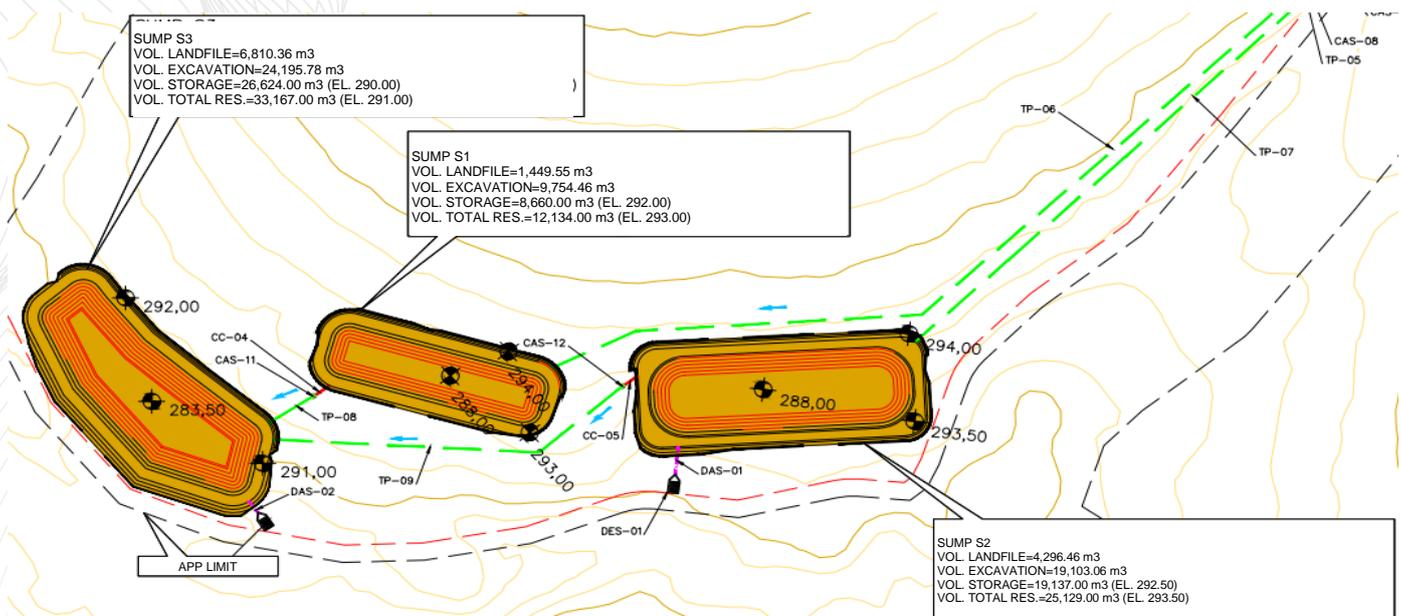
Figure 18-24 - Plant volume of sumps drainage sterile stockpile - PDE (GHT, 2022)
