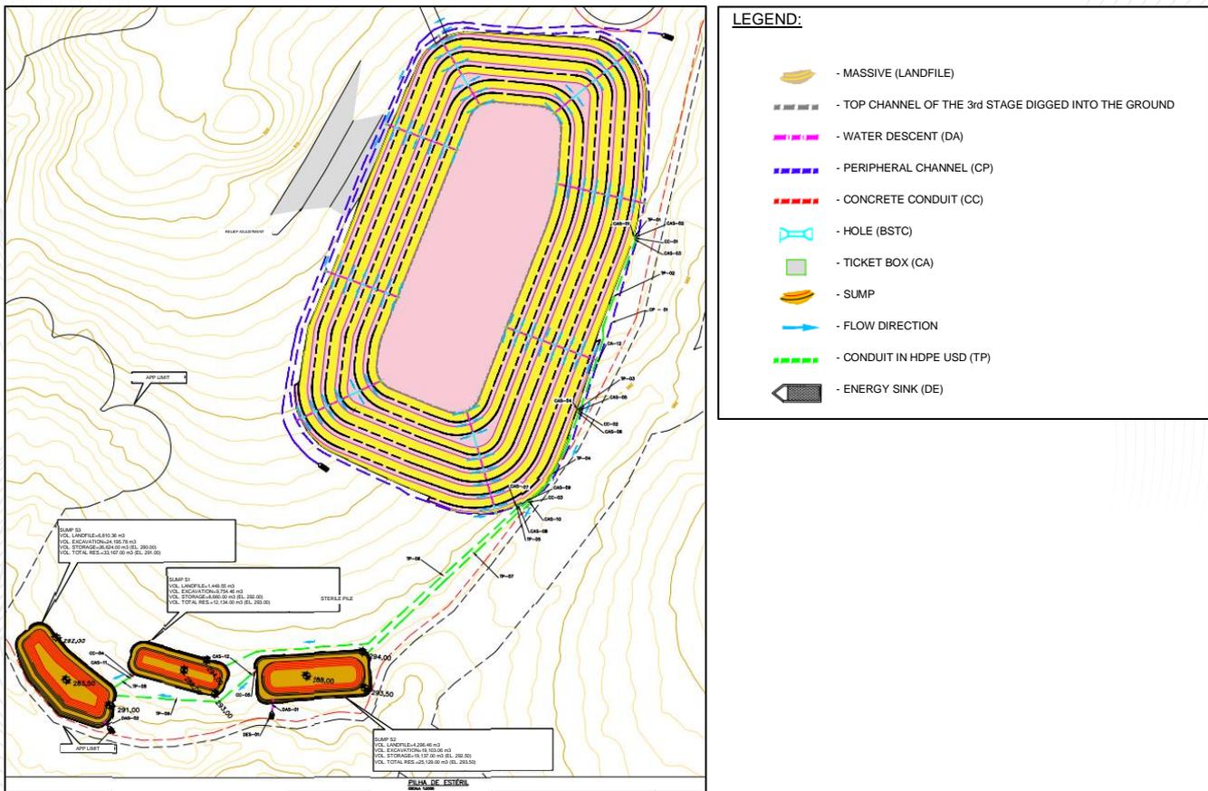
Figure 18-23 - Plant lease of sumps drainage sterile stockpile - PDE (GHT, 2022)
