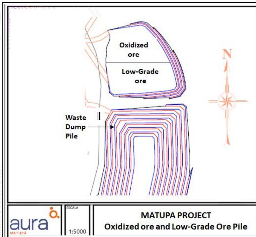
Figure 15-19 - Low-Grade and Oxidized Ores Schematic Stockpile Design.
