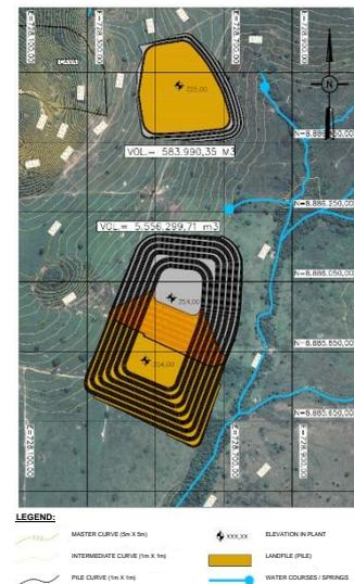
Figure 18-6 - Second year until the end of the fourth year of operation (MTP-B-DS-5010-GHT-G-0004, GHT, 2022)
