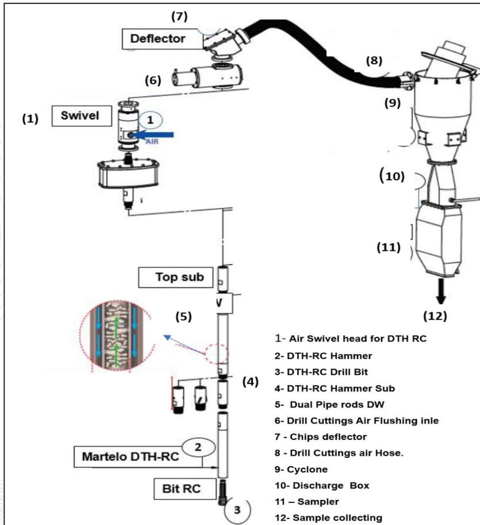
Figure 16-4 - Shows all the Main Components that Complement the Drilling Rig to Covert in RC Machine for Grade Control.
