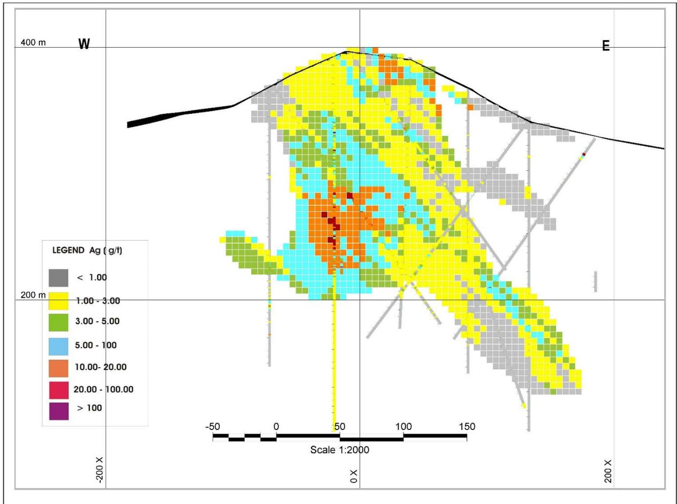
Figure 14-24 - Typical Cross-Section Through the X1 block Model Estimated Grades (Ag) (Looking N).
