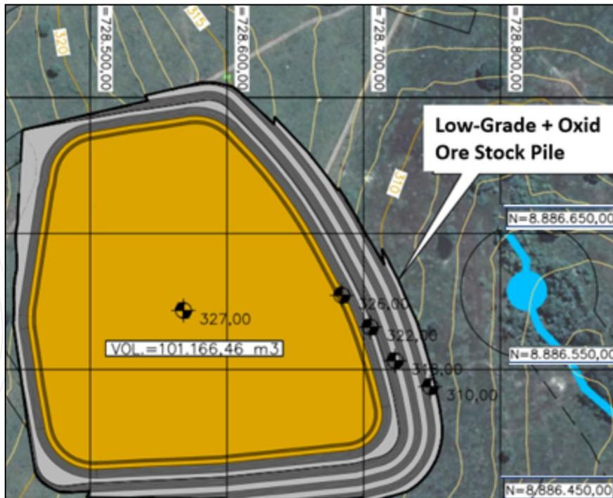
Figure 15-20 - Oxidized Ore + Low-Grade Ore Stockpile Design.
