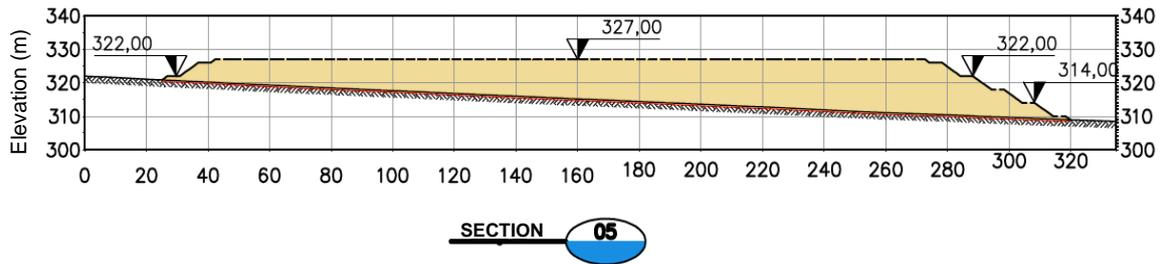
Figure 18-11 - Section 05 slope stability for the PMBT stockpiles (MTP-B-DS-5010-GHT-G-0013 - GHT, 2022)
