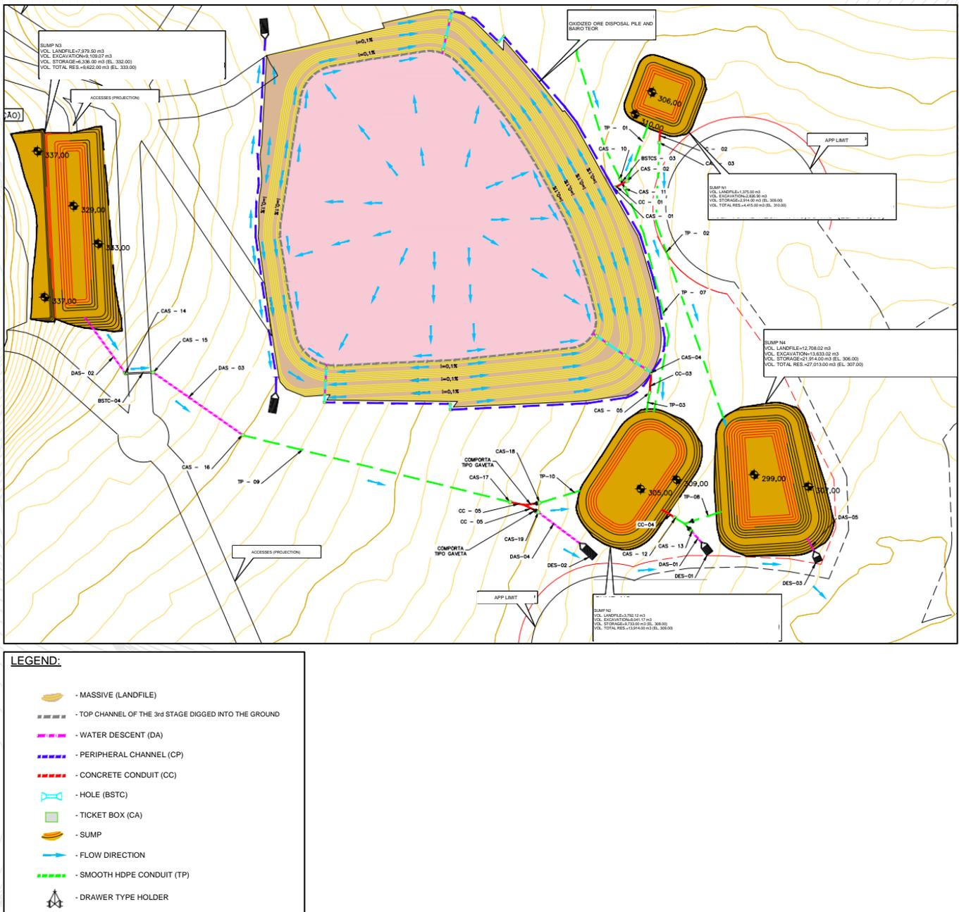
Figure 18-25 - Volume and lease plant of sumps drainage Low Grade Ore stockpile - PMBT (GHT, 2022)
