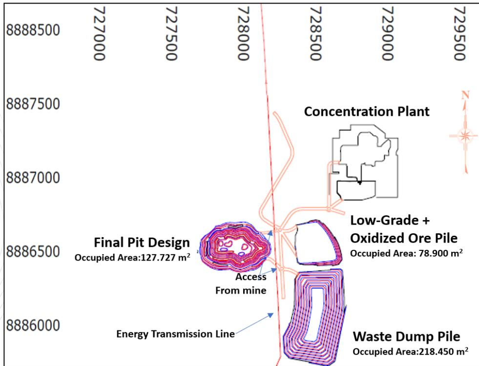
Figure 15-9 - General Layout Including Final Waste Dump Pile, Oxidized Ore and Low-Grade Ore Pile and Final Pit Design.
