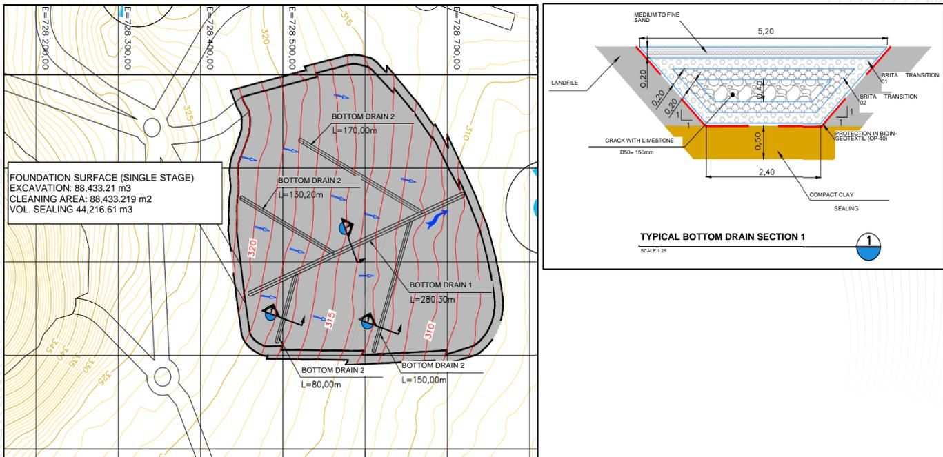
Figure 18-22 - Plant deep drainage Low Grade Ore stockpile - PMBT (GHT, 2022)
