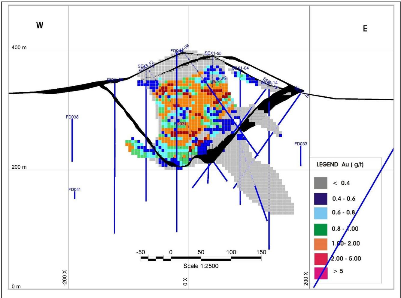
Figure 14-30 - Typical Cross-Section Through the X1 Block Model Estimated Grades (Au) showing resource pit outline in black. Looking N).
