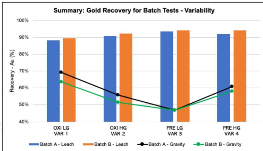
Figure 1-1 - Summary of Testing Results – Gravity/Leaching - Variability.
