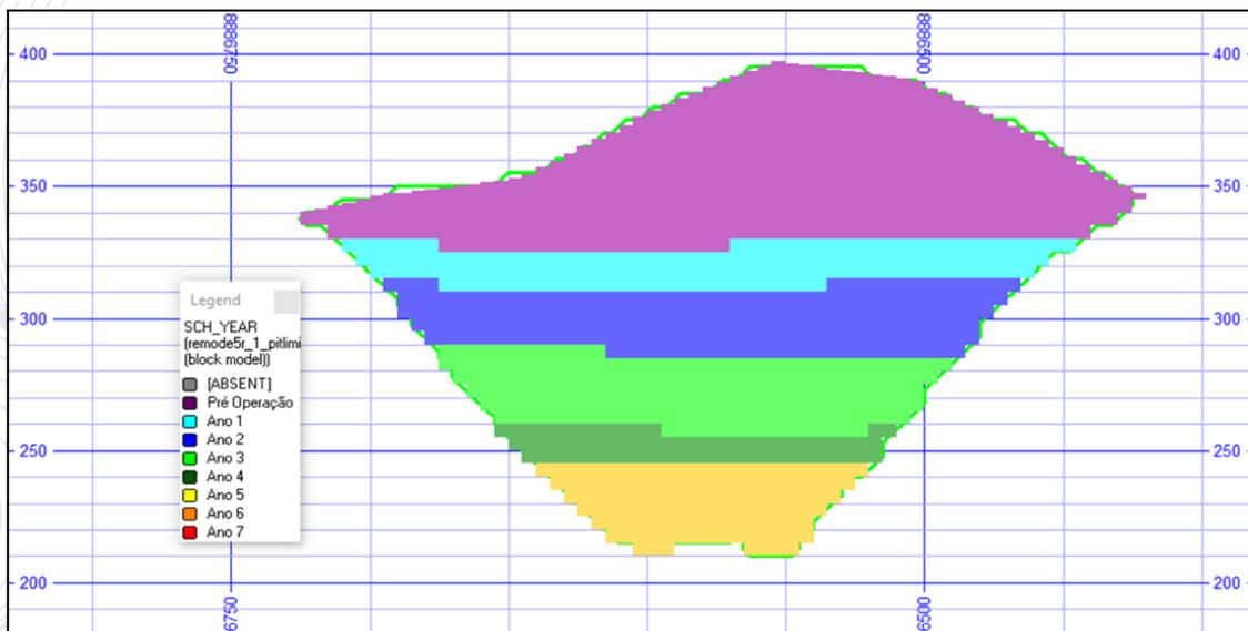
Figure 15-8 - A-A Profile Vertical CrossSection from the Open Pit Design (Figure 15.5).
