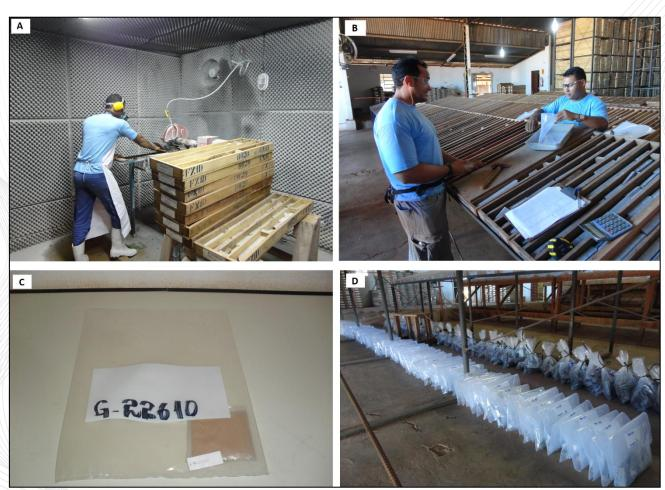
A) Core cutting facility in Rio Novo core-shack; B) Diamond drill core sampling at core-shack; C) Insertion of control samples; D) Samples inserted in tagged plastic bags.
