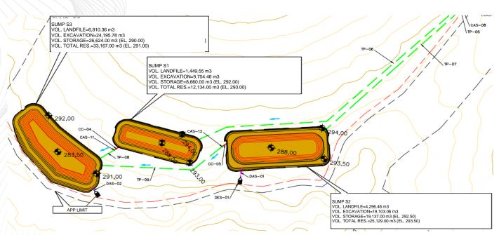
Figure 18-24 - Plant volume of sumps drainage sterile stockpile - PDE (GHT, 2022)
