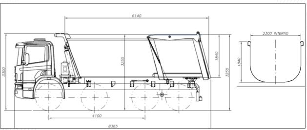
Figure 16-6 - Schematic Drawing of the 8 x 4 Truck with typical Bucket for Rossetti Mining Operations.
