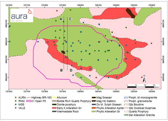
Note: Coordinates are South American Datum (1969), UTM Zone 21 South. Figure 7-23 - Diamond Core Drilling at X1 Deposit.
