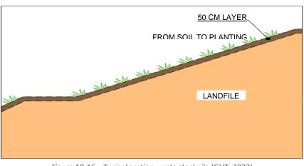
Figure 18-16 – Typical section waste stockpile (GHT, 2022)
