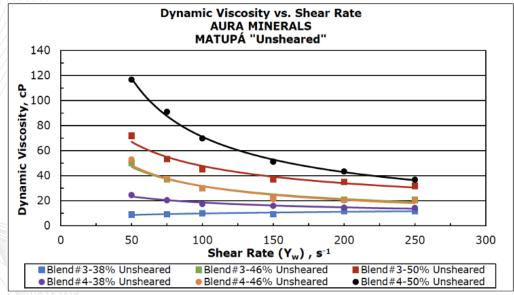
Figure 13-29 – Dynamic Viscosity as a Function of the Shear Rate - Third Campaign.
