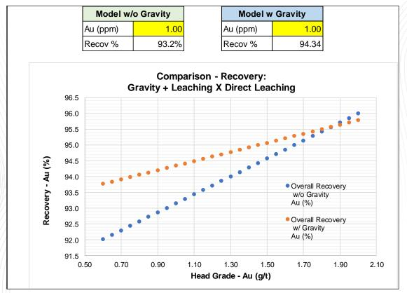
Figure 15-1 - Matupá Project Metallurgical Recovery Model After Consolidations Tests.
