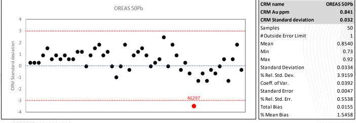
Figure 11-12 - Standard (50Pb) Sample Sequence Chart.
