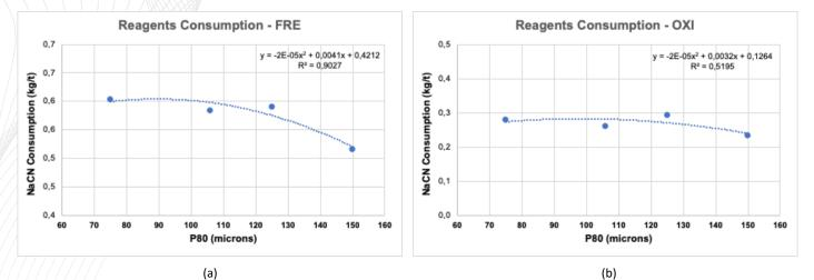
Figure 13-10 - Summary of NaCN Consumption in Leaching - CIL 24 h: (a) Fresh Rock; (b) Oxide Ore.
