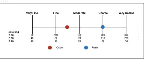
Figure 13-6 - Amira Scale for Gravity Tests (E-GRG).
