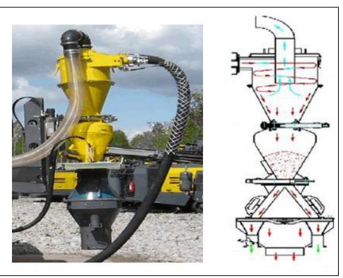
Figure 16-5 - Conical Sampler Illustration, Normally Recommended for Grade Control in Surface Mining Operations.
