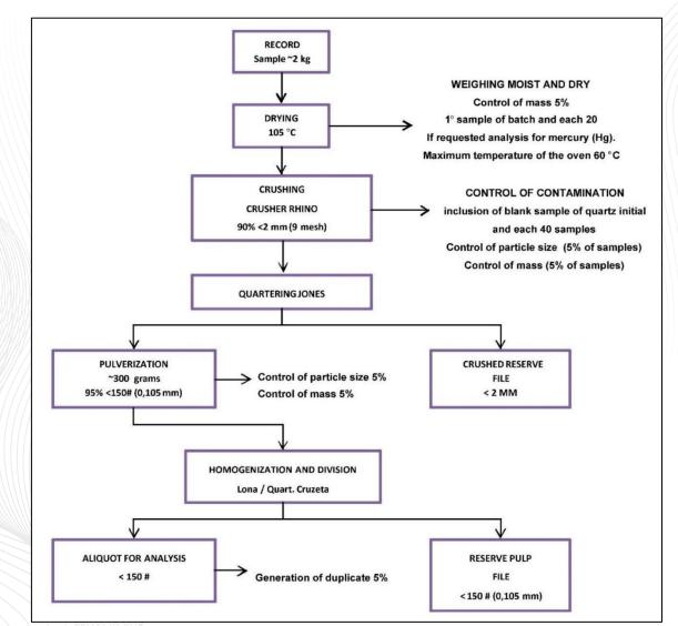
Figure 11-3 - Sample Preparation Protocol – Rock and Core (Rio Novo 2010-2012).
