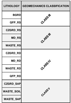
Table 15-8 - Geotechnics' Classification to the Rock Masses for the X1 Mineral Deposit.
