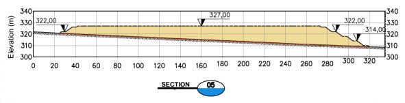
Figure 18-11 - Section 05 lope stablity for the PMBT stockpiles (MTP-B-DS-5010-GHT-G-0013 - GHT, 2022)
