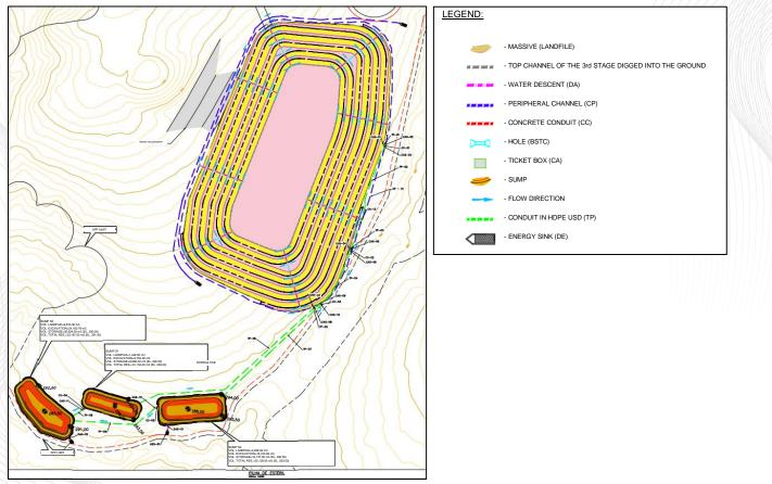
Figure 18-23 - Plant lease of sumps drainage sterile stockpile - PDE (GHT, 2022)
