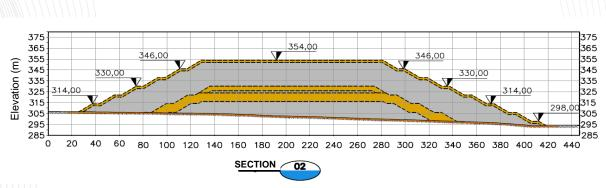
Figure 18-12 - Section 02 slope stablitiy for the PMBT stockpiles (MTP-B-DS-5010-GHT-G-0013 - GHT, 2022)
