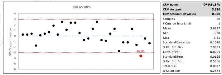
Figure 11-11 - Standard (18Pb) Sample Sequence Chart.
