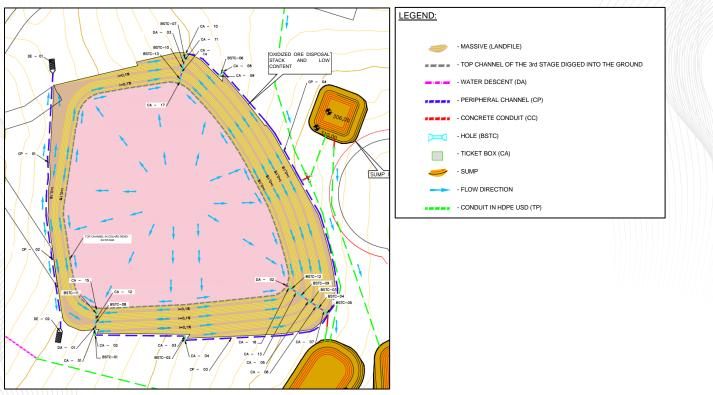
Figure 18-20 - Plant surface drainage Low Grade Ore stockpile - PMBT (GHT, 2022)
