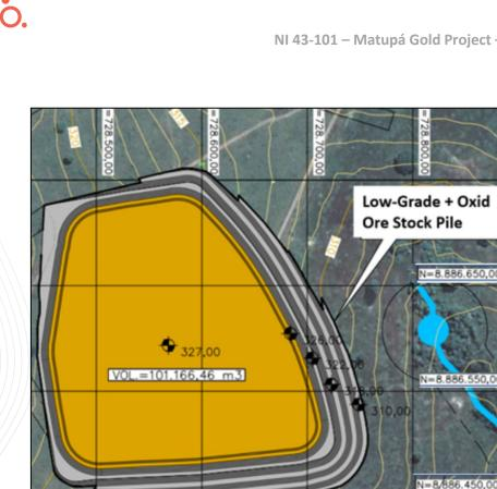
Figure 15-20 - Oxidized Ore + Low-Grade Ore Stockpile Design.
