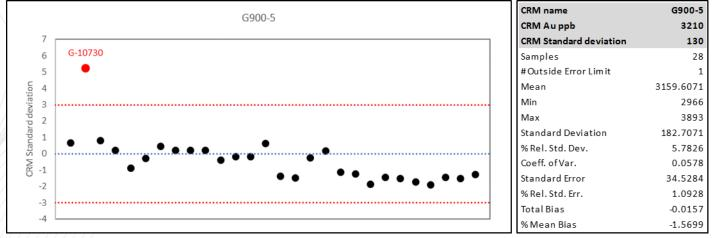
Figure 11-20 - Standard (G900-5) Sample Sequence Chart.
