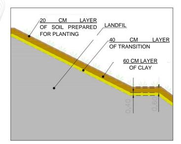
Figure 18-8 – Typical section with transition layer overlaid by clay with low degree, permeability and planting grasses
