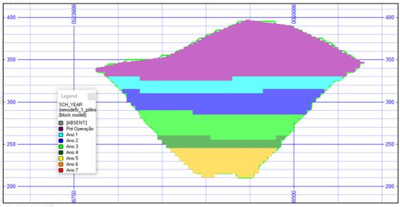
Figure 15-8 - A-A Profile Vertical CrossSection from the Open Pit Design (Figure 15.5).
