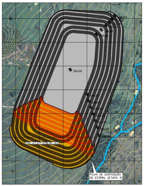
Figure 15-22 - Waste Dump Pile for the End of LOM.
