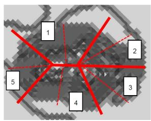
Figure 15-2 - Sectors Defined in X1 Typical Pit and the Sections for the Stability Analysis.
