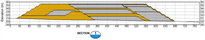
Figure 18-10 - - Section slope stablity for the PDE stockpiles (MTP-B-DS-5010-GHT-G-0013 - GHT, 2022)
