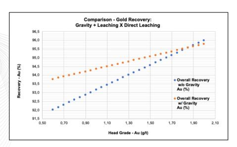
Figure 1-2 - Gold Recovery for Direct Leaching and Gravity/Leaching Routes - Consolidation.
