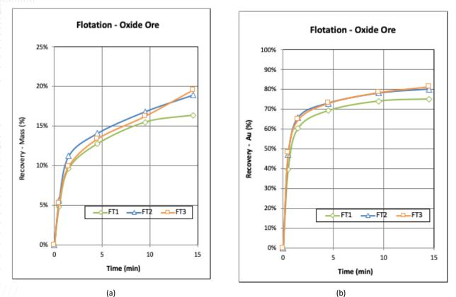
Figure 13-8 - Rougher Flotation - Oxide Ore: (a) Mass Recovery; (b) Gold Recovery.
