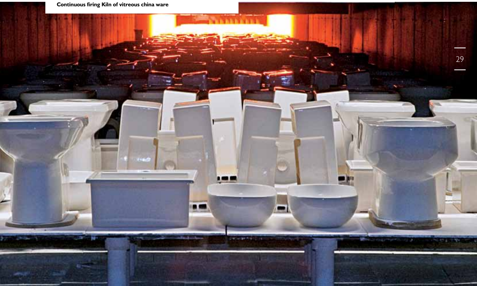
Continuous firing Kiln of vitreous china ware
