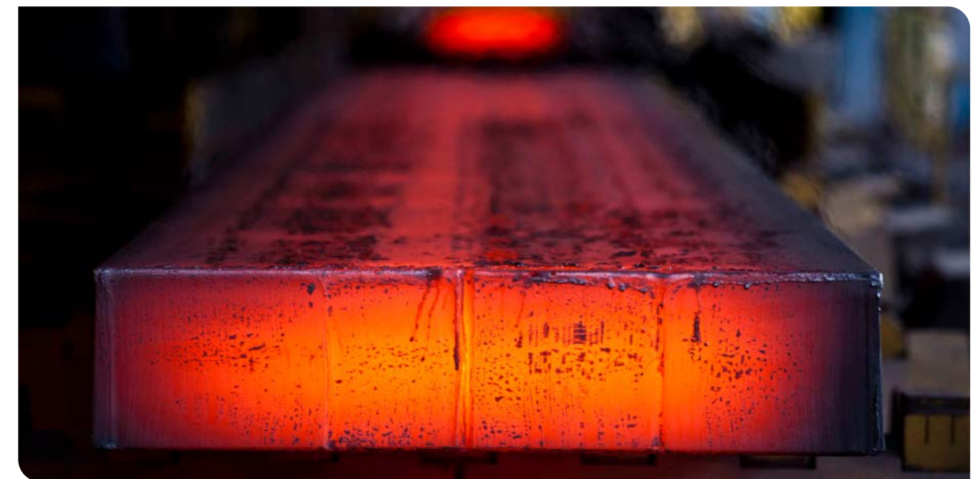
Steel plate in the hot rolling line at Presidente Vargas Steelworks in Volta Redonda
