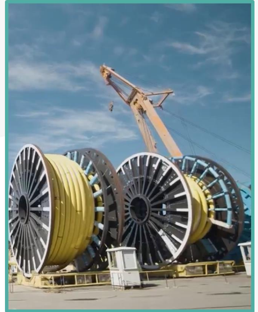
Spools with the tieback's flexible lines, before deployment
