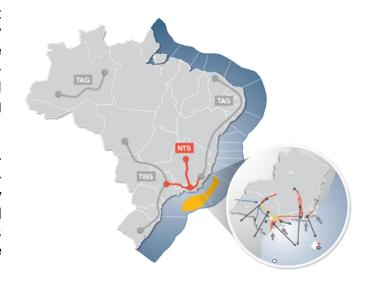
NTS's network has strong interconnection between its gas pipelines, connecting to the national production coming mainly from the Campos and Santos basins, the Bolivia-Brazil pipeline, owned by Transportadora Brasileira Gasoduto Bolívia-Brasil (TBG), the gas pipelines in the Northeast region of Brazil, owned by Transportadora Associada de Gás (TAG), and the Guanabara Bay LNG terminal, owned by Petrobras, totaling nine points for receiving and 47 points for delivering gas in the region.
