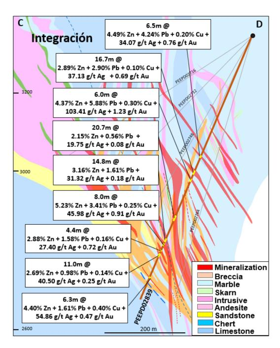
In 4Q24, we will continue drilling the south extension of the Integración target at the 3,300 level, aiming to further extend the mineralization. A total of 1,800 meters is planned with one rig.
