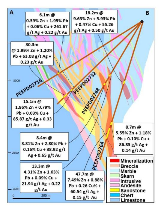
For 3Q24, we plan to continue drilling the southern extension of the Integración target at 3,300 level, aiming to extend the mineralized zone (1,800 meters with three rigs).
