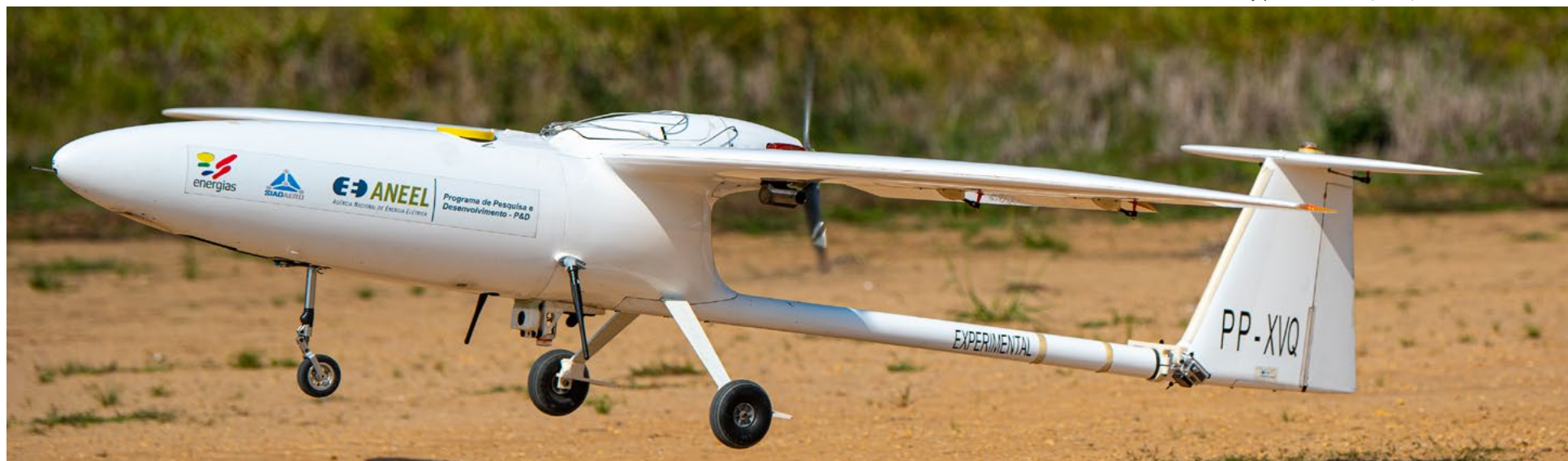
Remotely piloted aircraft (RPAs) for network monitoring.
