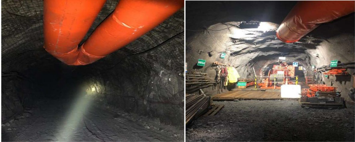
Figure 13-12: Ventilation Ducting Used to Ventilate Work Headings
