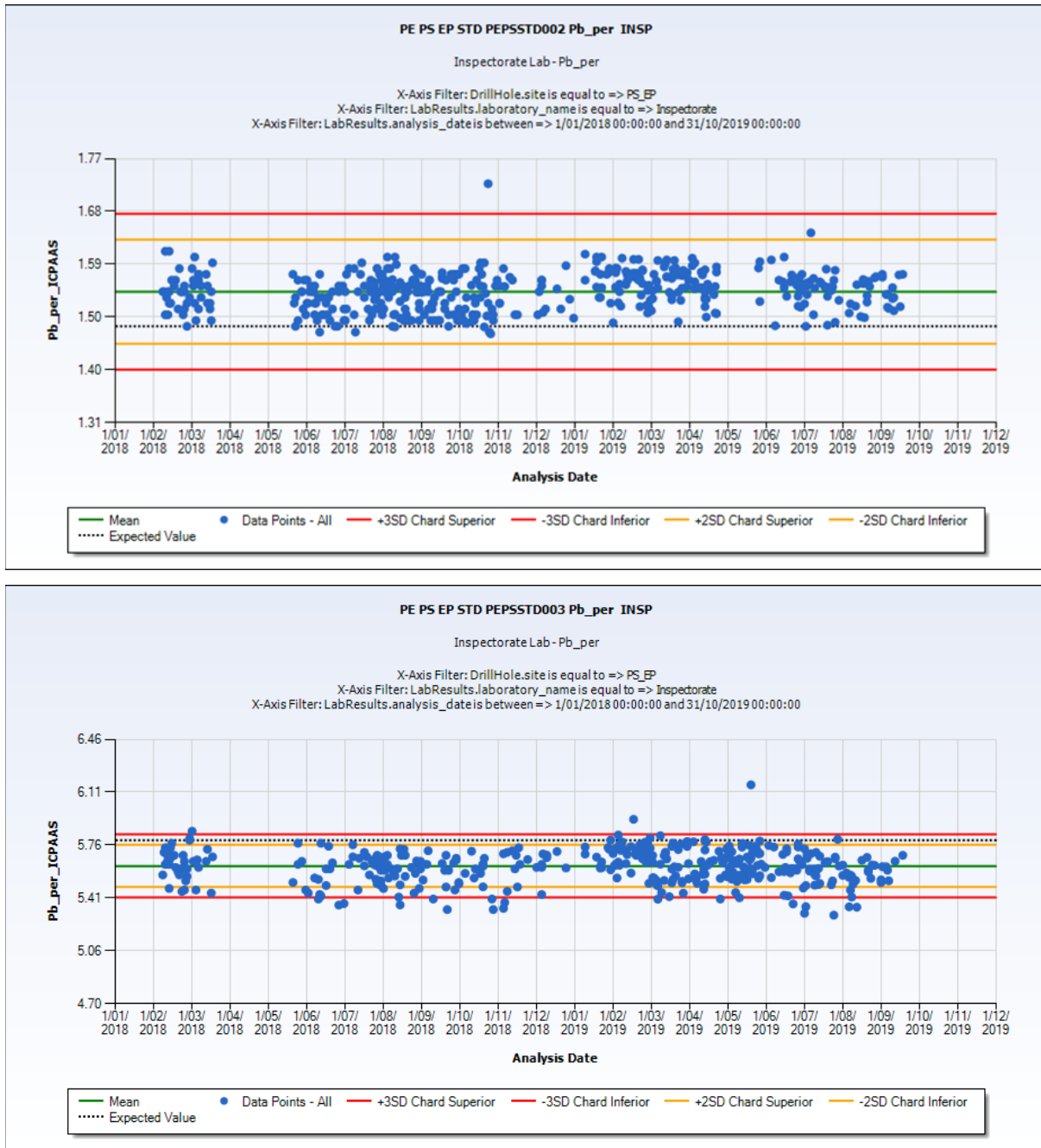
Figure 8-4: CRMs PEPST002 and PEPST003 Results for Lead –Inspectorate EP (2018 to 2019)
